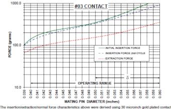
and polished steel gauge pins having a bullet-shaped tip. The curves represent typical average values: they are best used to compare the differences between similar size
