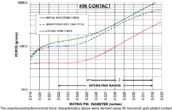
and polished steel gauge pins having a bullet-shaped tip. en similar size
