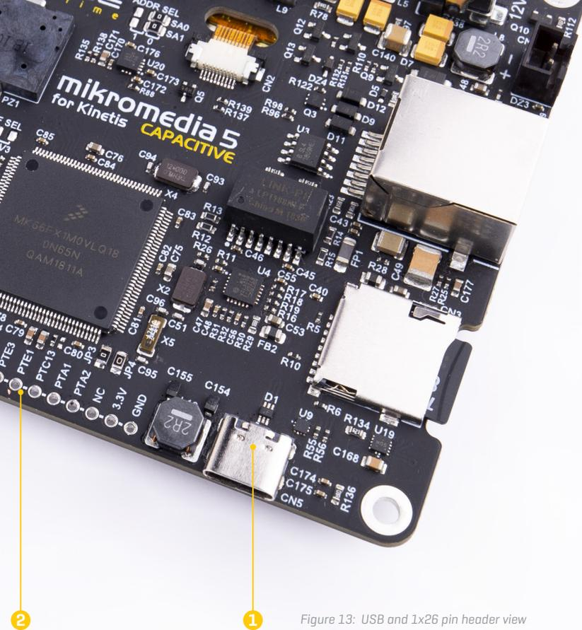
Figure 13: USB and 1x26 pin header view
