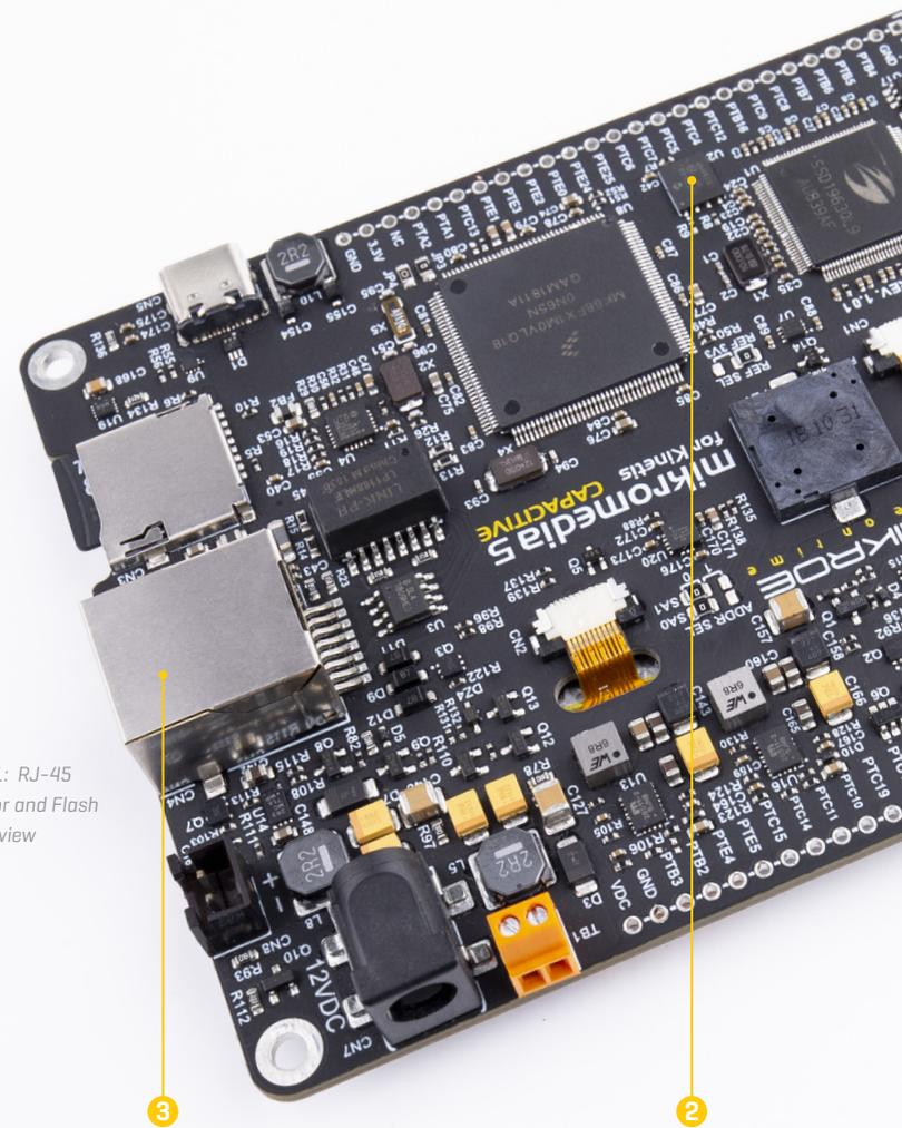
Figure 11: RJ-45 connector and Flash memory view
