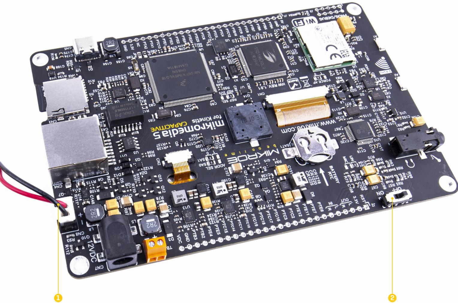
Figure 8: Battery power supply connection
