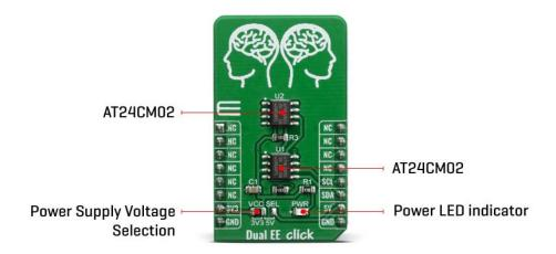
This Click board™ uses the I2C communication protocol. Therefore, every data transaction event is initiated by the host MCU, transmitting the I2C START condition, followed by the AT24CM02 device ID byte. Upon receiving the device ID byte, the AT24CM02 IC expects two more address bytes, completing the 18bit address word.
