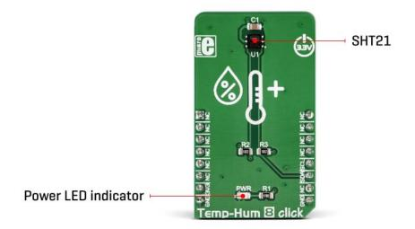
The SHT21 IC is based on the CMOSens® technology, featuring the capacitive RH sensor and the bandgap temperature sensor. Besides the sensing elements, the IC incorporates an analog front end (AFE), which consists of A/D converter, OTP memory, and a logic section. The integrated
