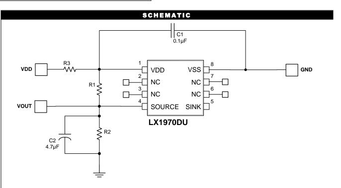
The LX1970 Mini Light Sensor Board can be used to convert a manual DC voltage dimmer to a closed loop automatic dimmer. The resistor values can be changed to fit the design requirements. The LX1970 output current is proportional to the incident light intensity up to the point where either the current source voltage compliance is exceeded or the light sensor saturates. See the data sheet and application note for additional information.
