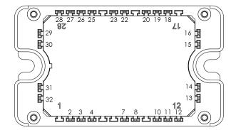
Pins 25 to 28 must be shorted together Pins 13 to 16 must be shorted together Pins 18/19/20/22 must be shorted together
