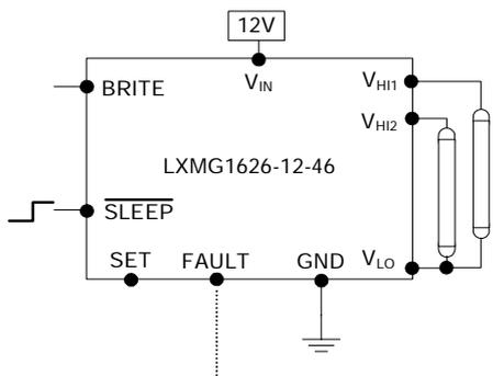
**Figure 2 – FAULT Output Operation**
