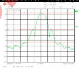
$V_C$  = 3.3V,  $V_{REF}$  = 2.95V,  $I_{CQ}$  = 65mA, Frequency = 2.45GHz
