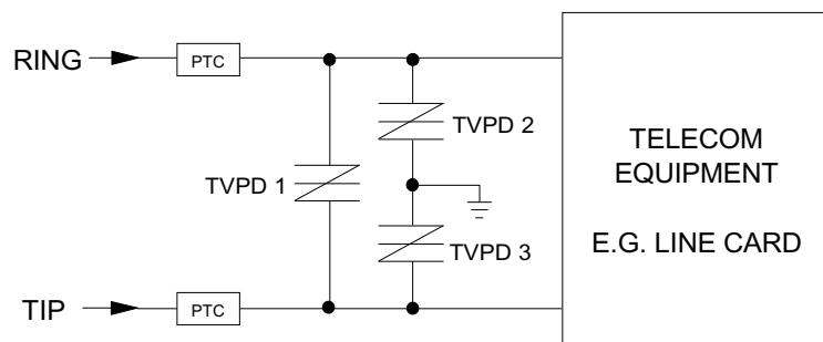
The PTC (Positive Temperature Coefficient) is an overcurrent protection device.
