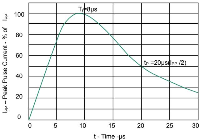
Fig 1. Pulse Waveform
