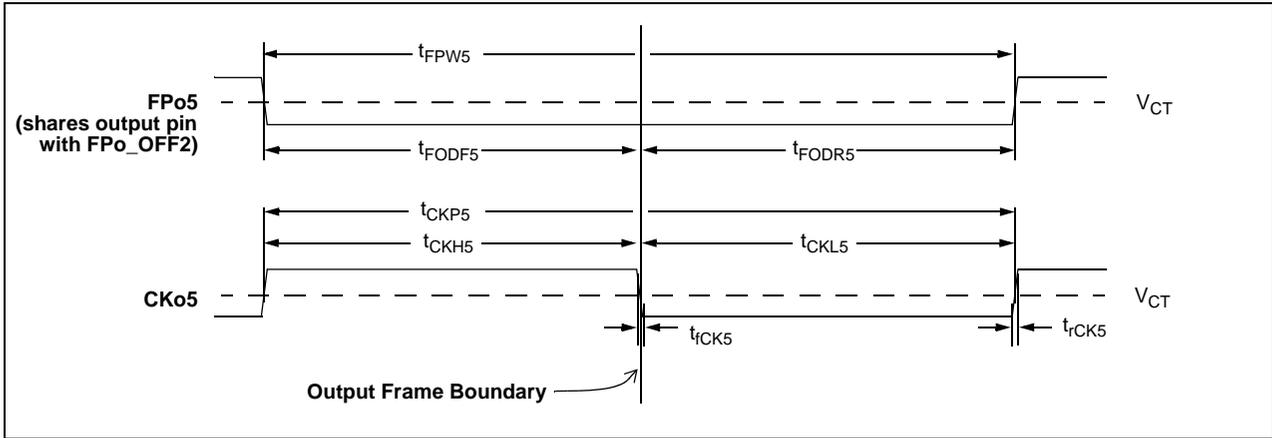
Figure 47 - CKo5 Timing Diagram (19.44 MHz)
