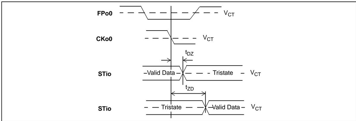
**Figure 39 - Serial Output and External Control**
