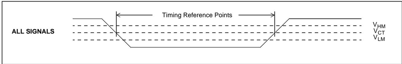
**Figure 25 - Timing Parameter Measurement Voltage Levels**
