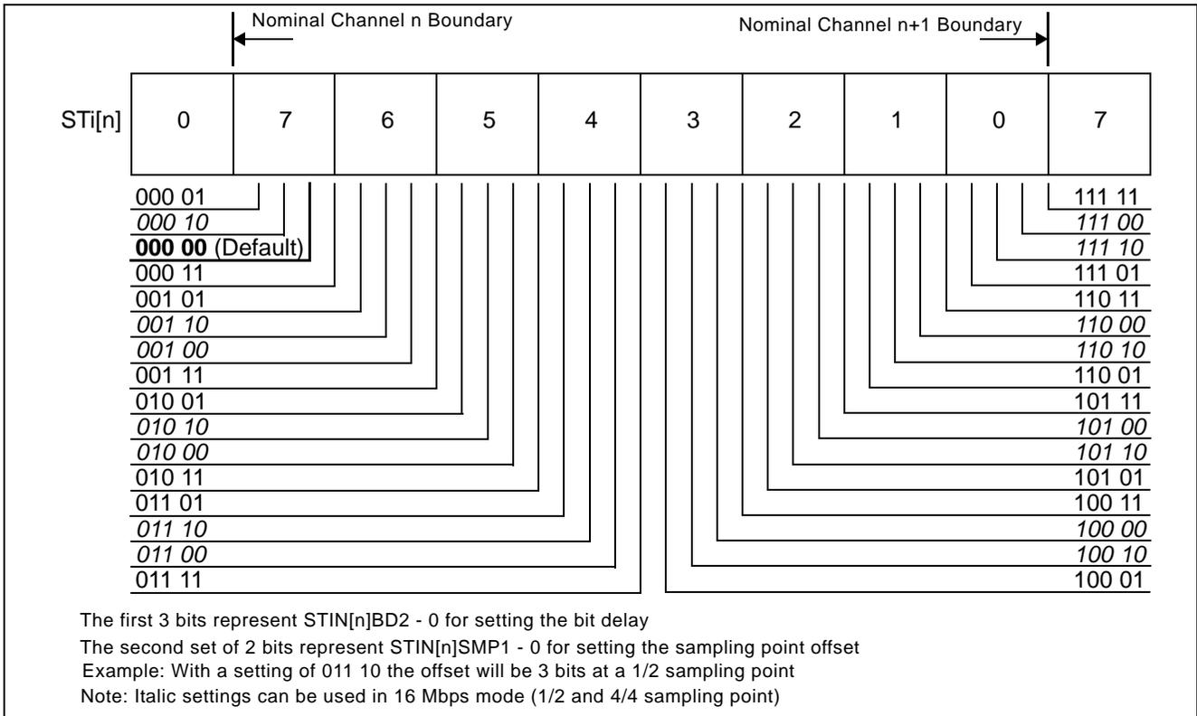
**Figure 15 - Input Bit Delay and Fractional Sampling Point**
