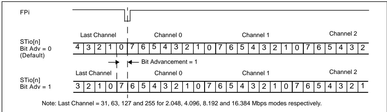
**Figure 16 - Output Bit Advancement Timing Diagram (ST-BUS)**
