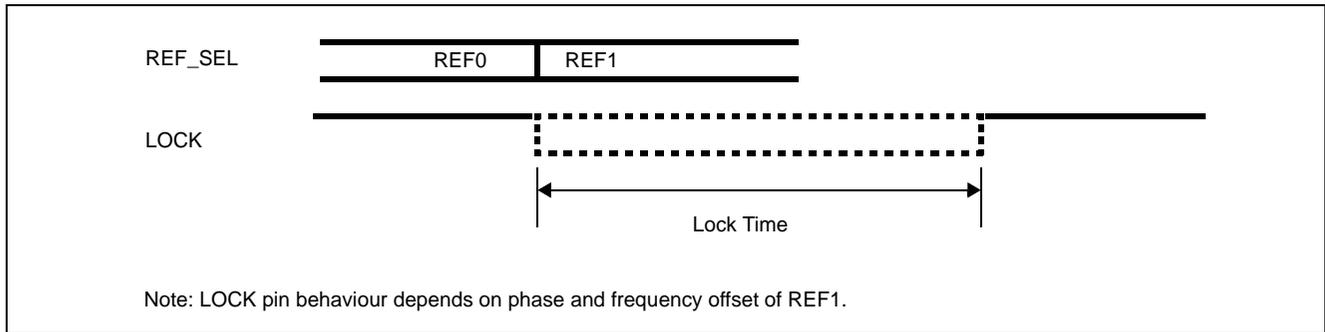
**Figure 10 - Reference Switching in Normal Mode**
