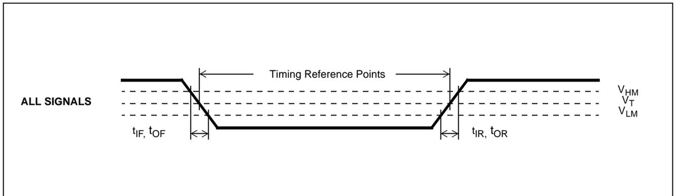
**Figure 14 - Timing Parameter Measurement Voltage Levels**
