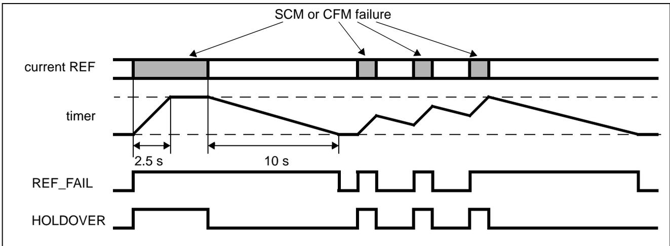
**Figure 4 - Behaviour of the Dis/Requalify Timer**
