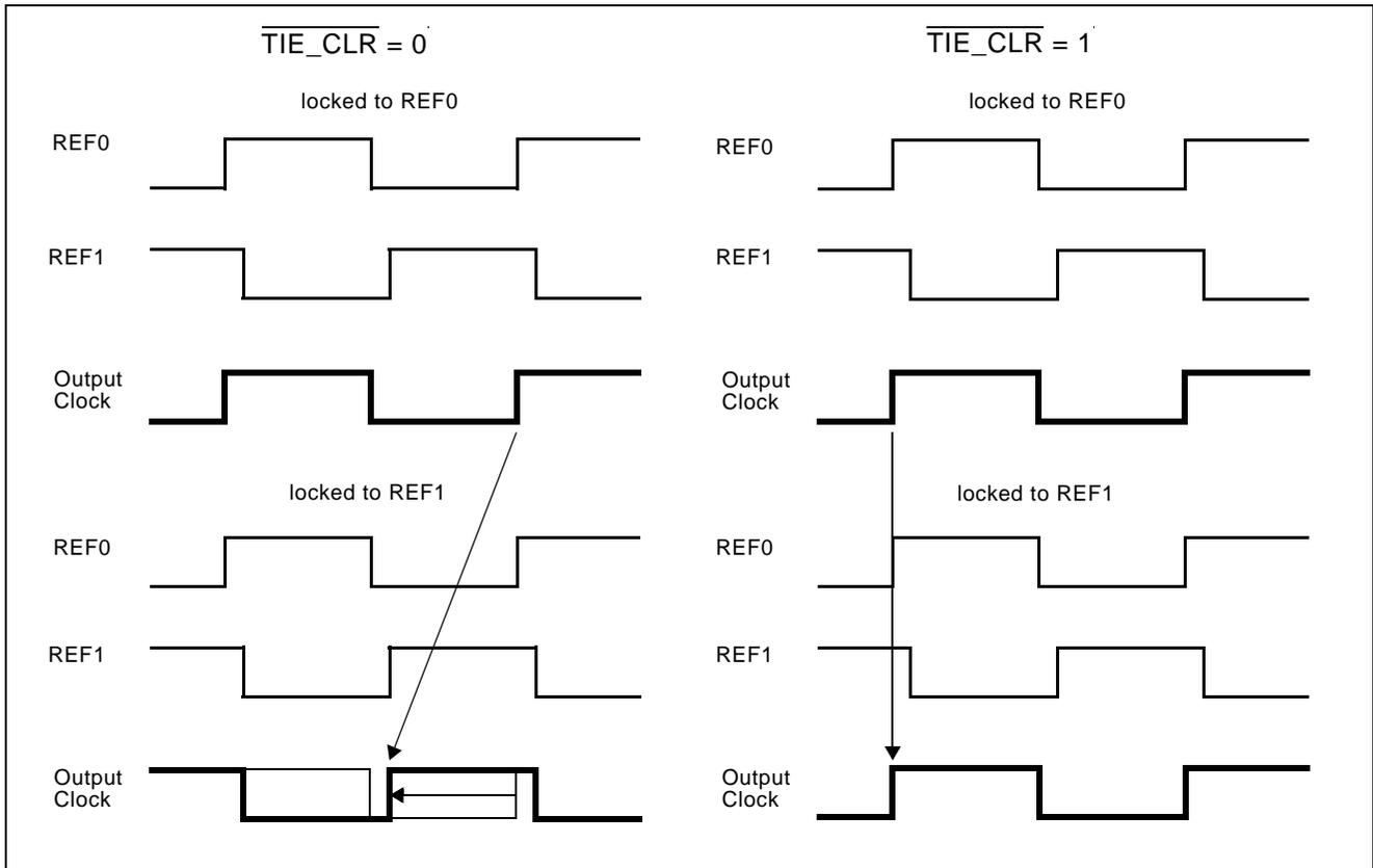
**Figure 6 - Timing Diagram of Hitless Reference Switching**
