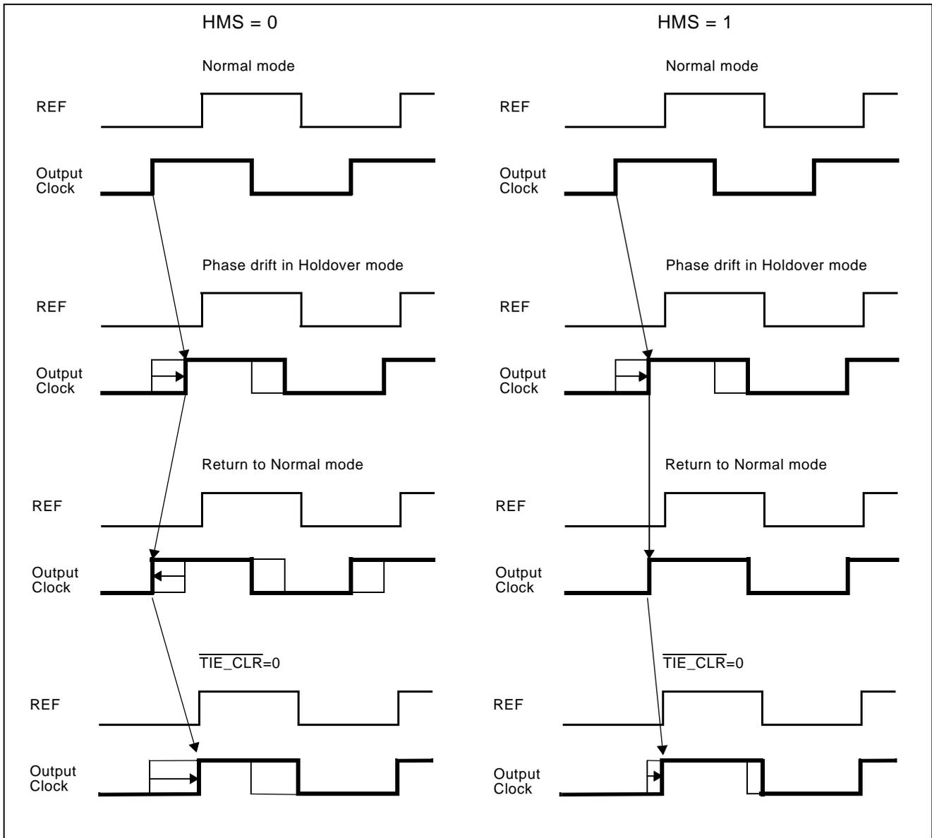
**Figure 7 - Timing Diagram of Hitless Mode Switching**
