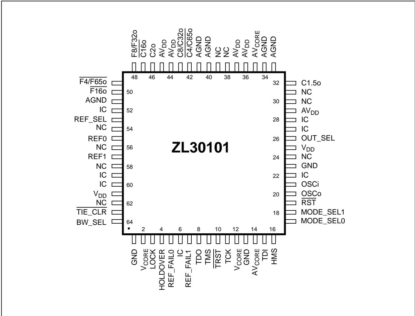
Figure 2 - Pin Connections (64 pin TQFP, please see Note 1)
