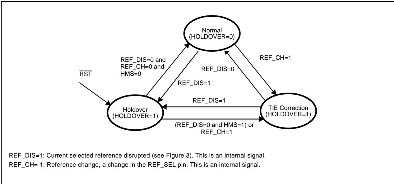
**Figure 9 - Mode Switching in Normal Mode**
