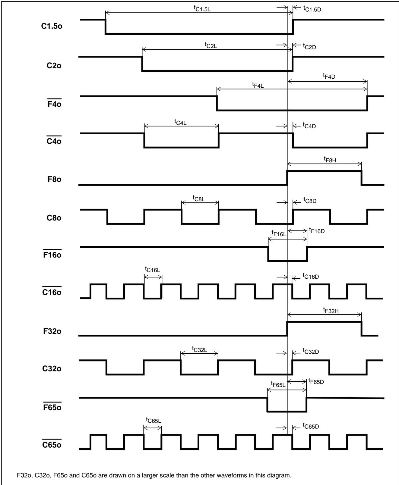
Figure 16 - Output Timing Referenced to F8/F32o
