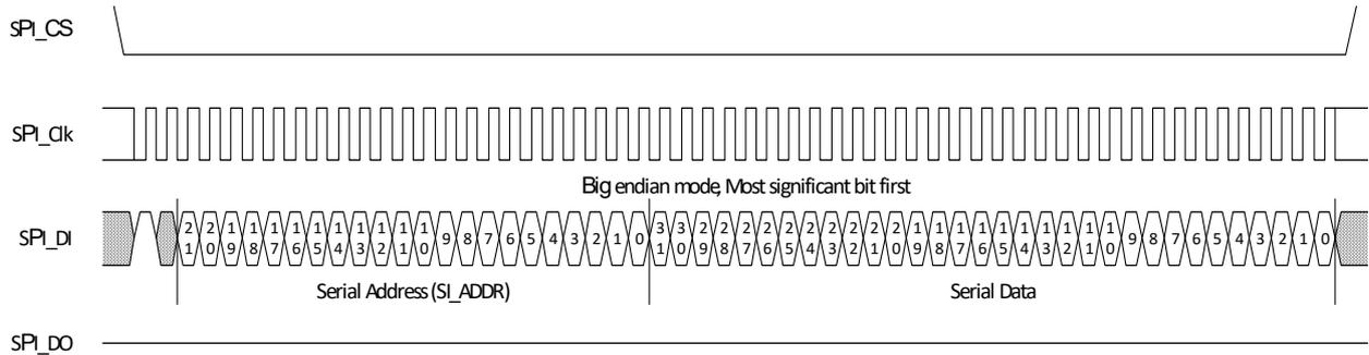
**Figure 54 • SPI Read Cycle**
