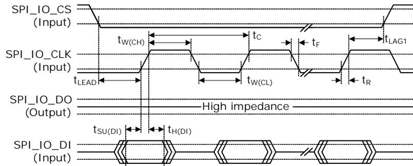
**Figure 76 • SI Output Data Timing Diagram for Slave Mode**
