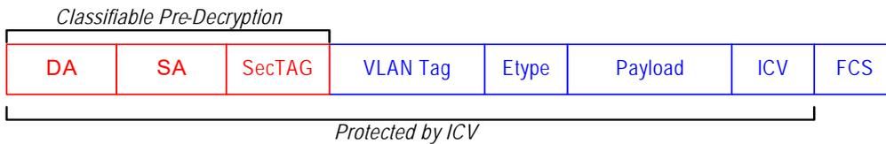
**Figure 26 • Dual-Tagged Ethernet**
