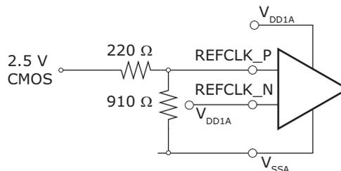
**Figure 48 • 3.3 V CMOS Single-Ended REFCLK Input Resistor Network**
