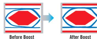
**VariSense**, which controls the USB receiver sensitivity enabling programmable levels of USB signal receive sensitivity. This capability allows operation in a sub-optimal system environment, such as when a captive USB cable is used.
