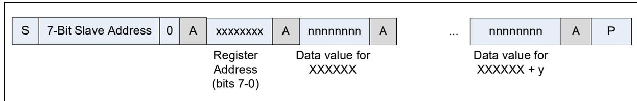
In this operation, following the 7-bit slave address, the 8-bit register address is written indicating the start address for sequential write operation. Every subsequent access is a data write to a data register, where the register address increments after each access and an ACK from the slave occurs. Sequential write access is terminated by a Stop condition.
