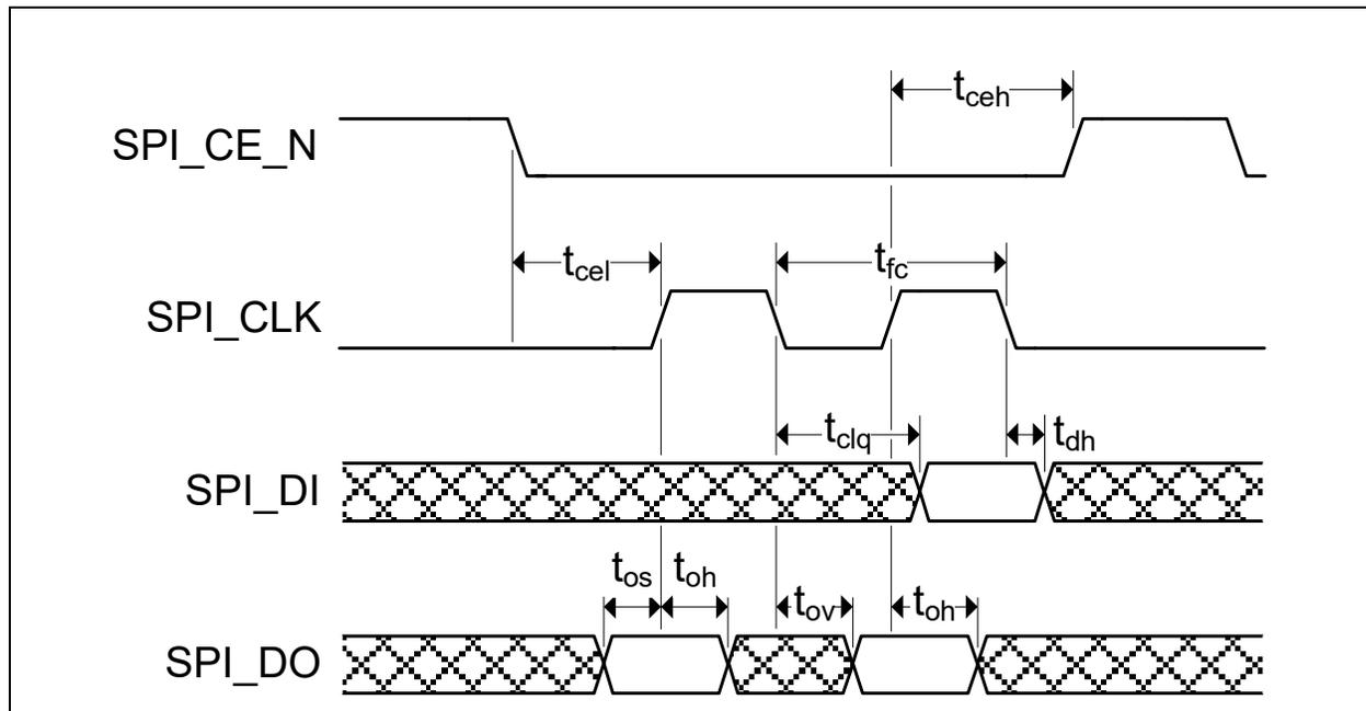
**Note:** The SPI can be configured for 30 MHz or 60 MHz operation via the `SPI_SPD_SEL` configuration strap. 30 MHz operation timing values are shown in [Table 9-9](#). 60 MHz operation timing values are shown in [Table 9-10](#).
