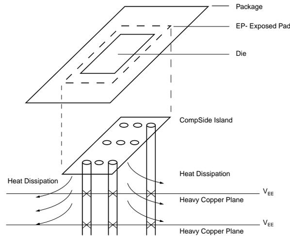
**PCB Thermal Consideration for 64-Pin EPAD-TQFP Package
