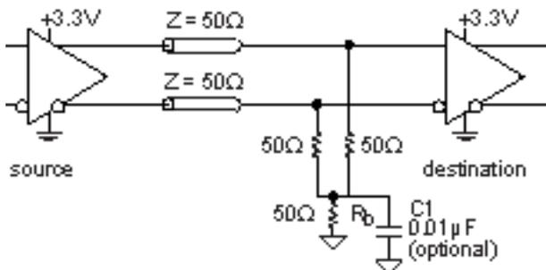
**Figure 5. Three-Resistor "Y-Termination"**
