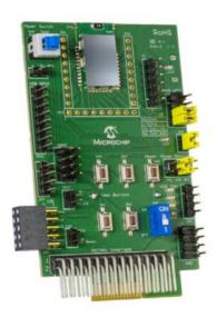
The RN-4870-SNSR is a development board based on the ultra-compact Bluetooth 4.2 Low Energy RN4870 module. The RN4870 uses a simple ASCII command interface over the UART. The board enables evaluation of the RN4870 and development of Bluetooth low Energy applications in two different ways:
