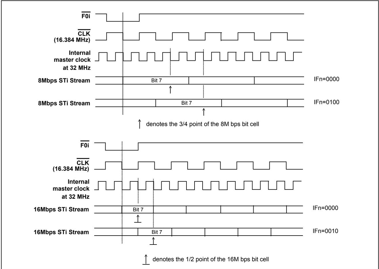
Figure 6 - Examples for Input Offset Delay Timing
