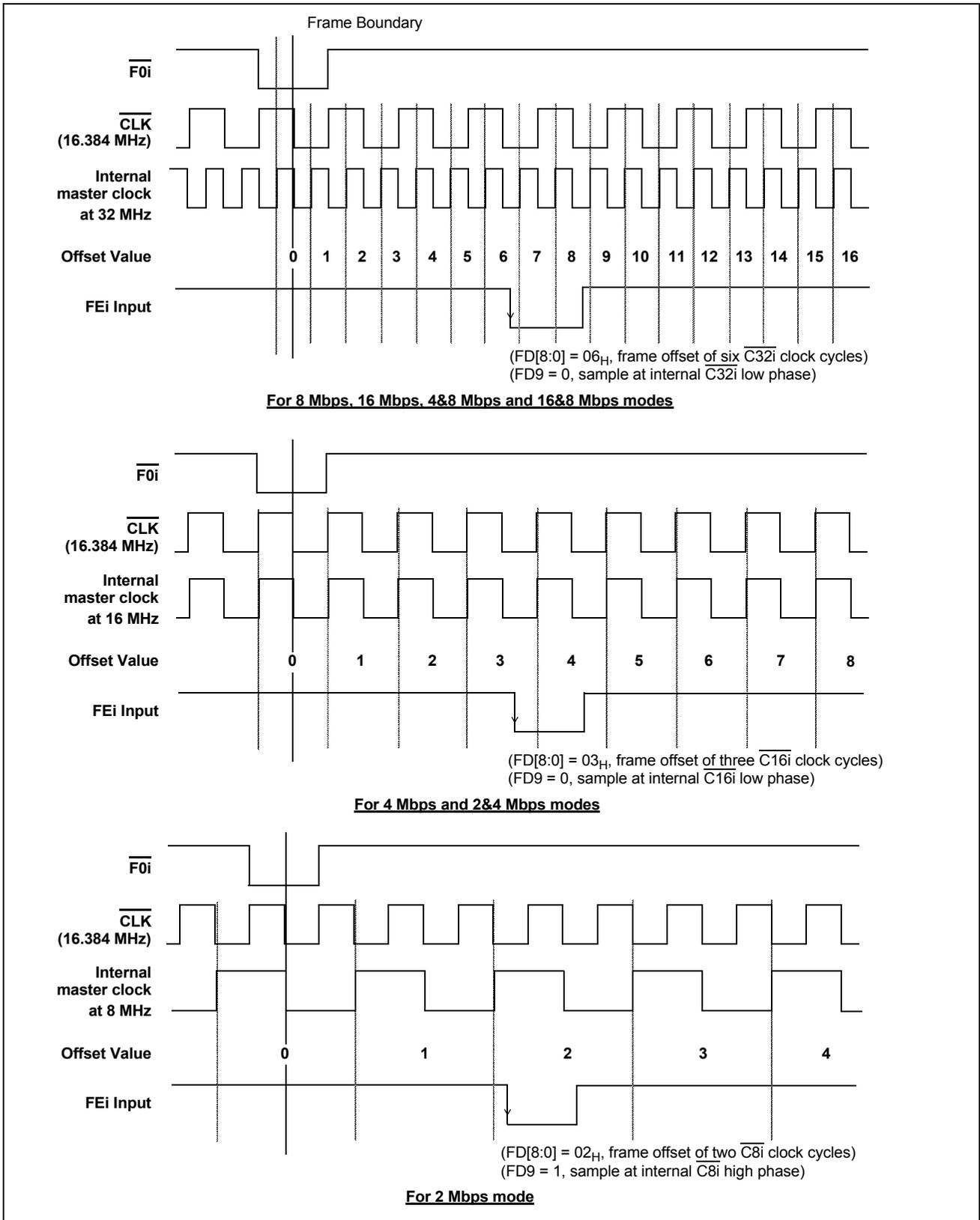
Figure 5 - Example for Frame Alignment Measurement
