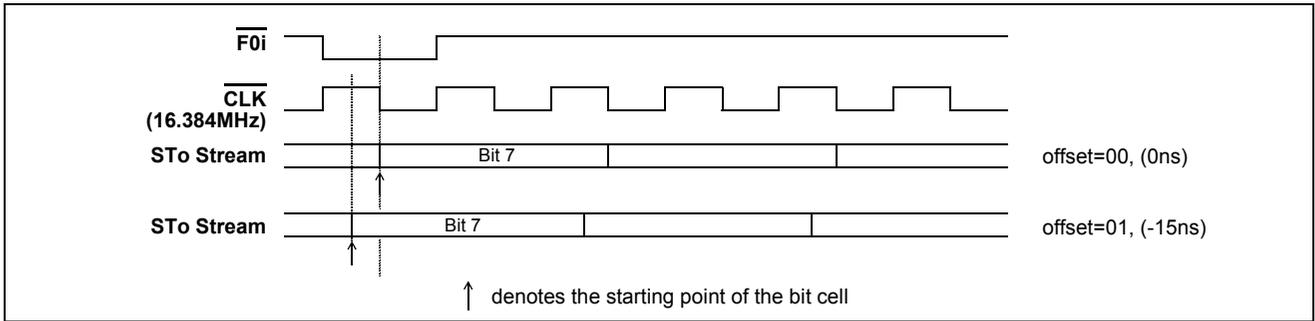
Figure 7 - Examples for Frame Output Offset Timing
