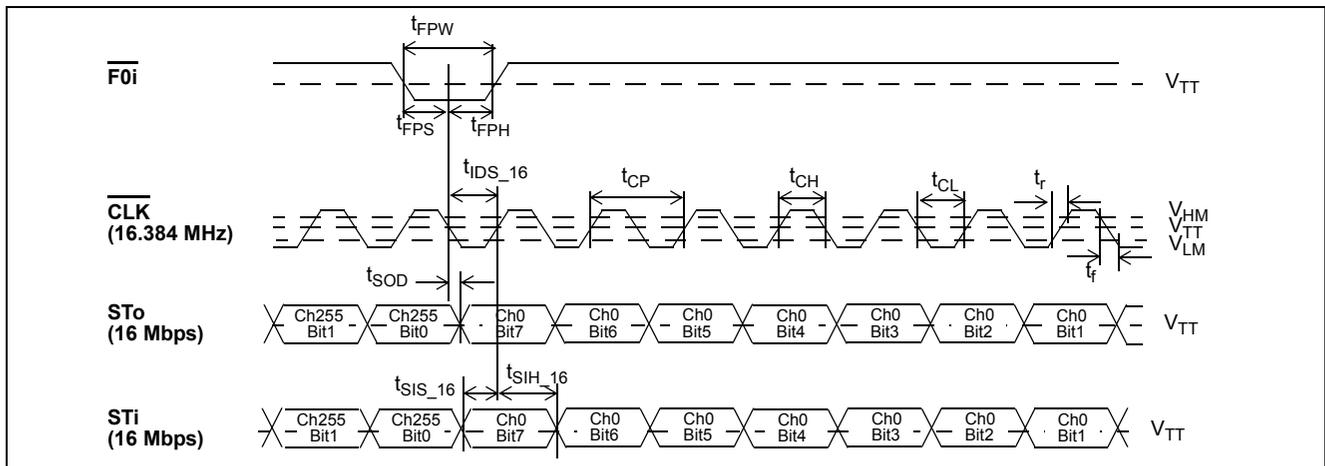
**Figure 8 - ST-BUS Timing for Stream rate of 16.384 Mbps**
