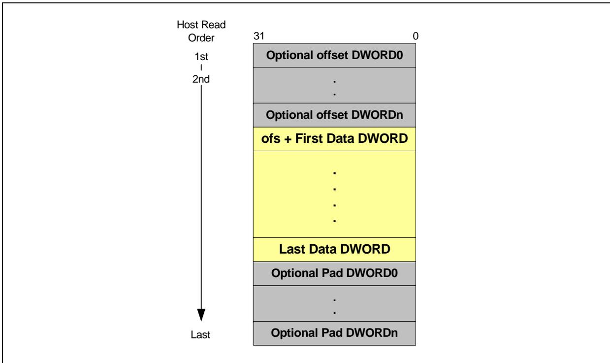
**Note 3-17** The LAN9217 host bus interface supports 16-bit bus transfers; internally, all data paths are 32-bits wide. [Figure 3-18](#) describes the host read ordering for pairs of atomic 16-bit transactions.
