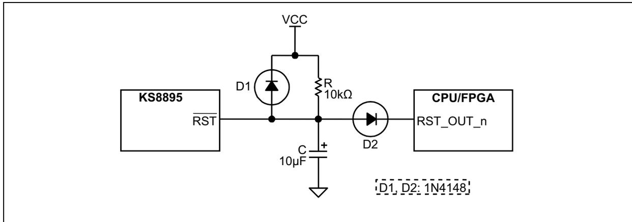
At power-on-reset, R, C, and D1 provide the necessary ramp rise time to reset the device. The reset out  $\text{RST\_OUT\_n}$  from CPU/FPGA provides the warm reset after power-up.
