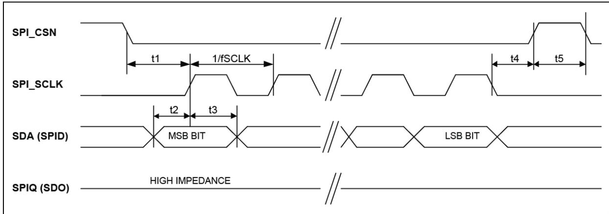
**FIGURE 7-10: SPI OUTPUT TIMING**
