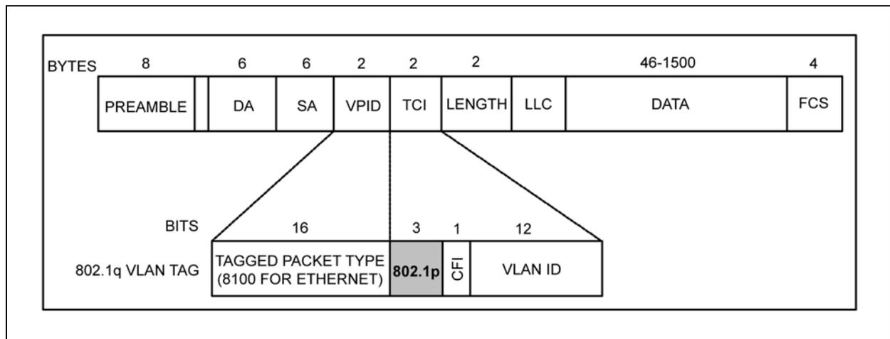
802.1p-based priority is enabled by bit [5] of the Registers Port Control 0 for ports 1, 2, 3, 4, and 5, respectively.
