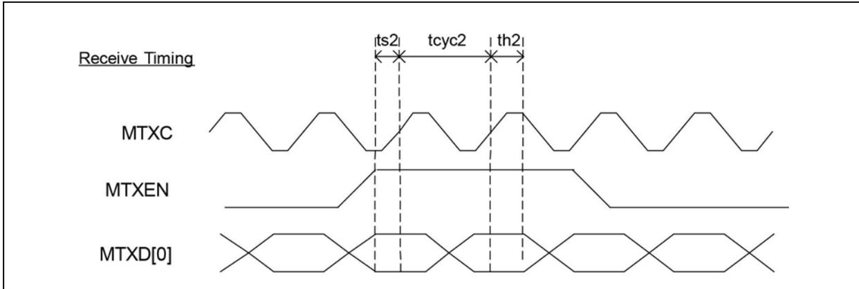
FIGURE 7-4: SNI OUTPUT TIMING
