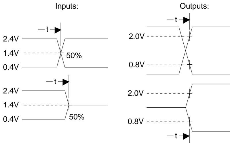
Inputs are driven at 2.4V for logic "1" and 0.4 V for logic "0" except XTAL1 pin.
