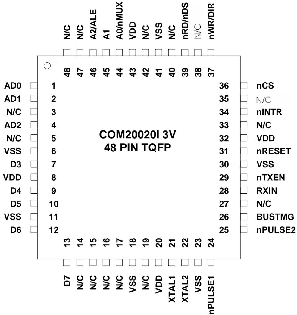
**NOTE: BUSTMG pin is only TQFP package**
