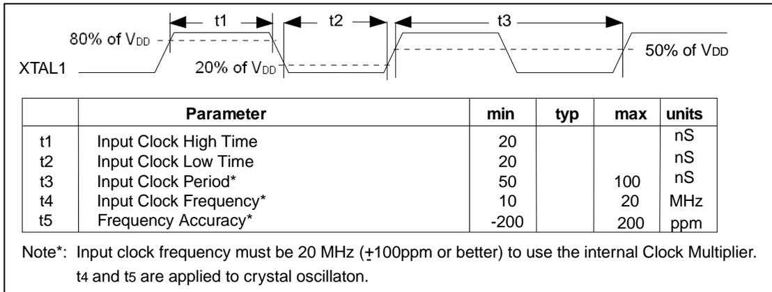
Figure 25 – TTL Input Timing On XTAL1 Pin
