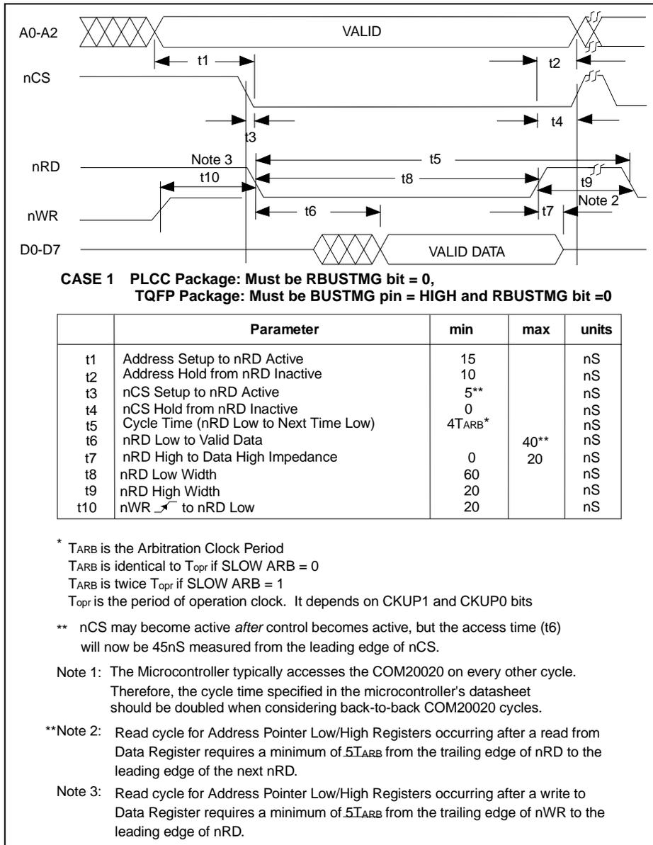
**Figure 15 - Non-Multiplexed Bus, 80xx-Like Control Signals; Read Cycle**
