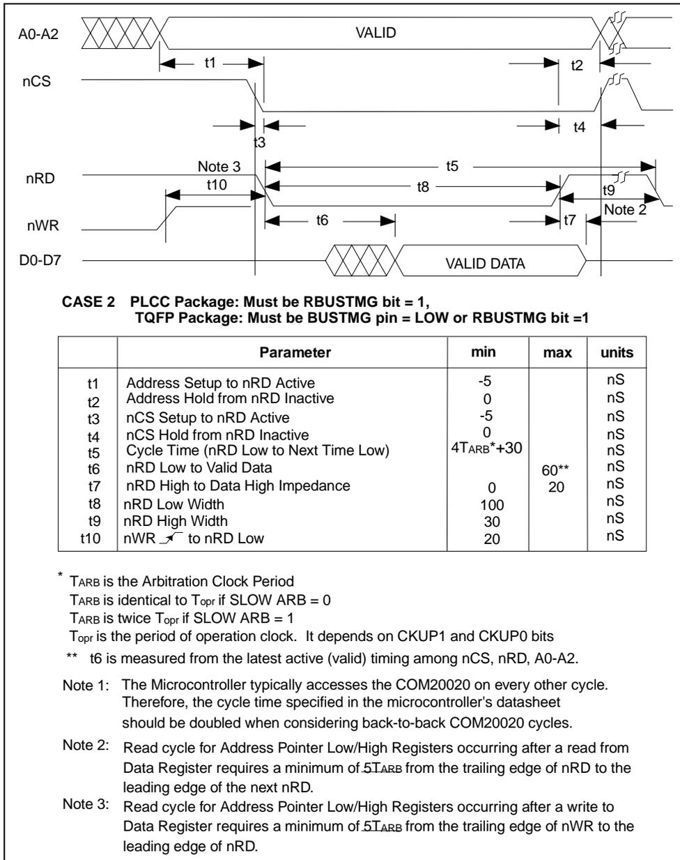
**Figure 16 - Non-Multiplexed Bus, 80xx-Like Control Signals; Read Cycle**
