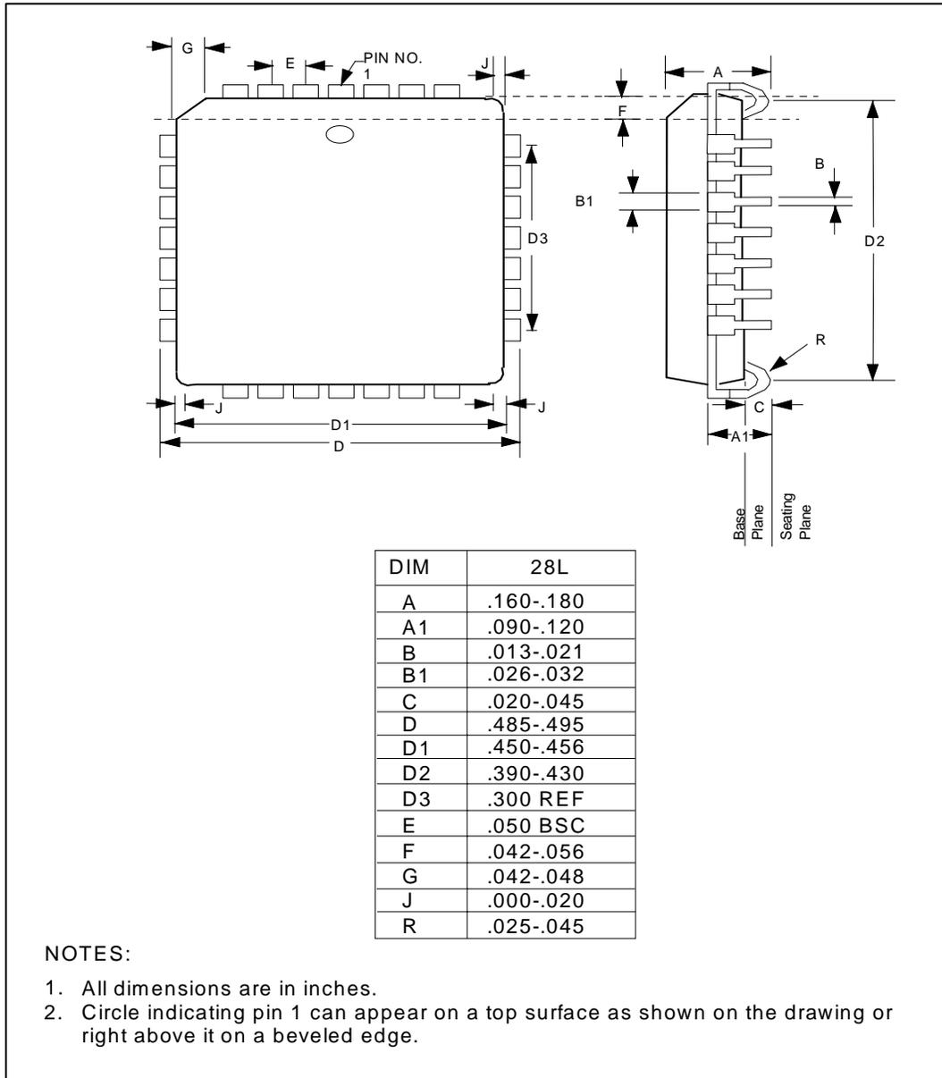
Figure 27 - 28 Pin PLCC Package Dimensions
