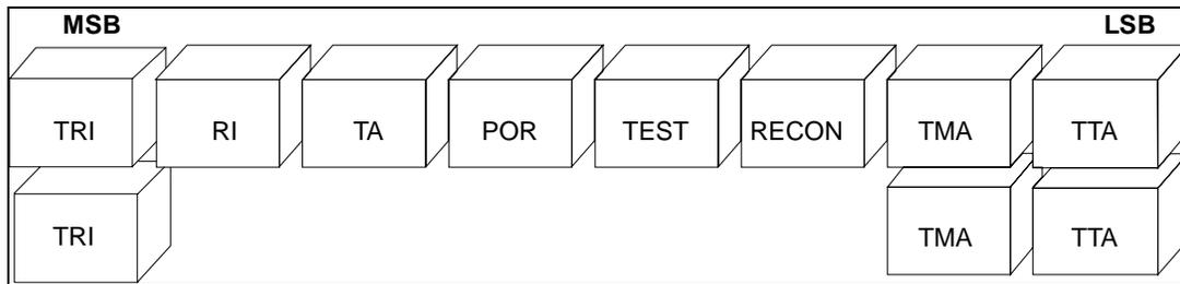
**Figure 10 - Command Chaining Status Register Queue**
