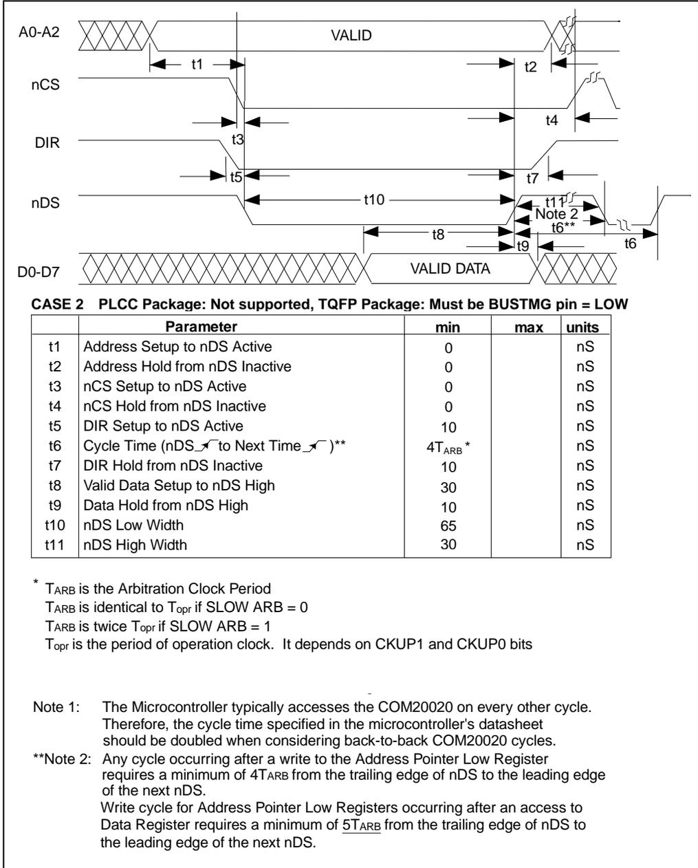
**Figure 22 - Non-Multiplexed Bus, 68xx-Like Control Signals; Write Cycle**
