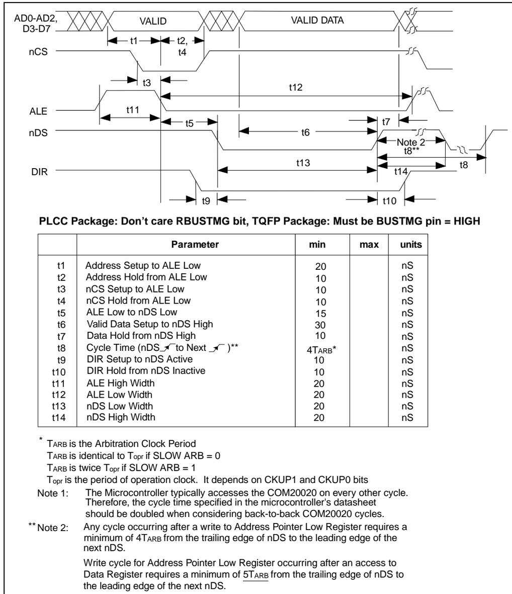
Figure 13 - Multiplexed Bus, 68xx-Like Control Signals; Write Cycle
