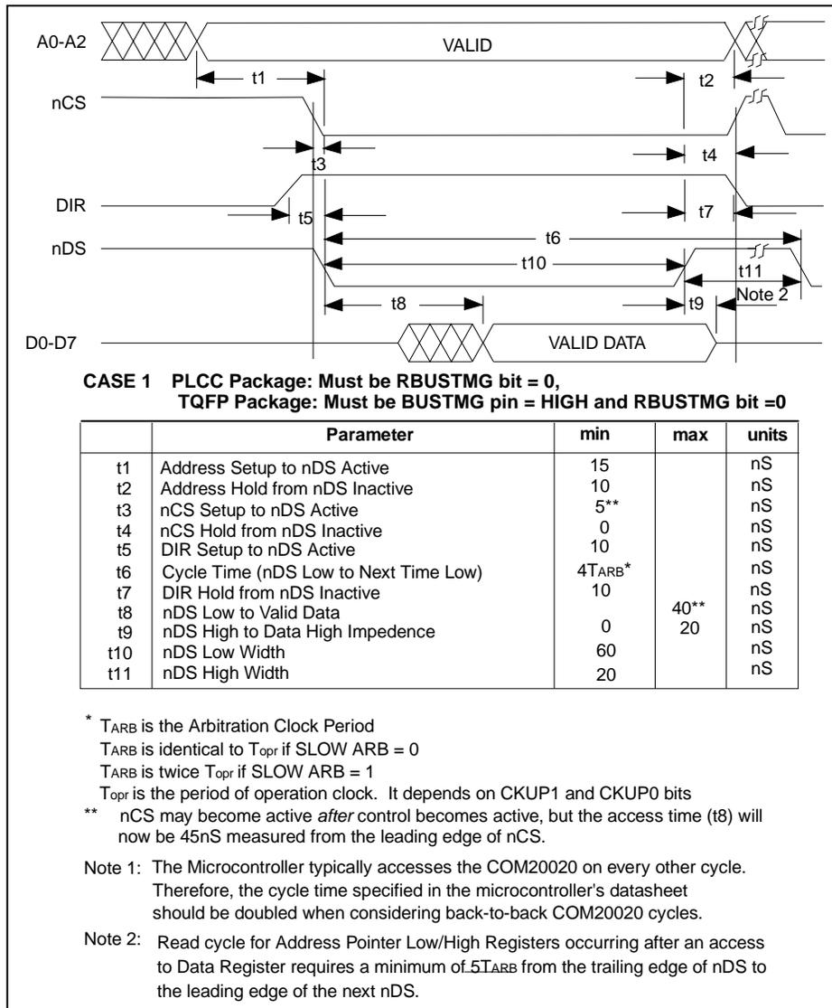
Figure 17 - Non-Multiplexed Bus, 68xx-Like Control Signals; Read Cycle
