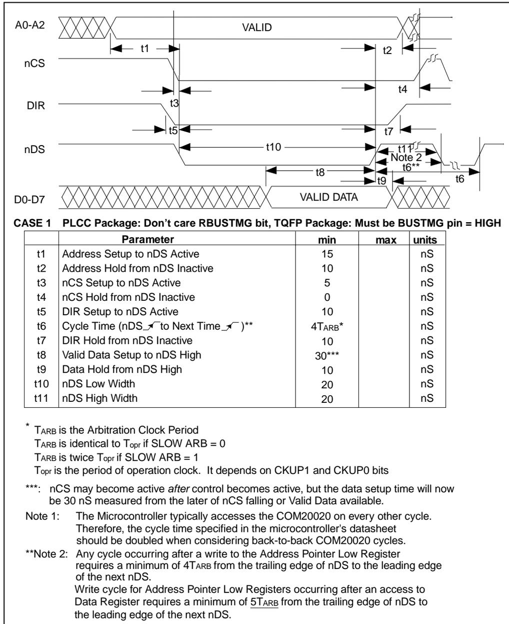
**Figure 21 - Non-Multiplexed Bus, 68xx-Like Control Signals; Write Cycle**
