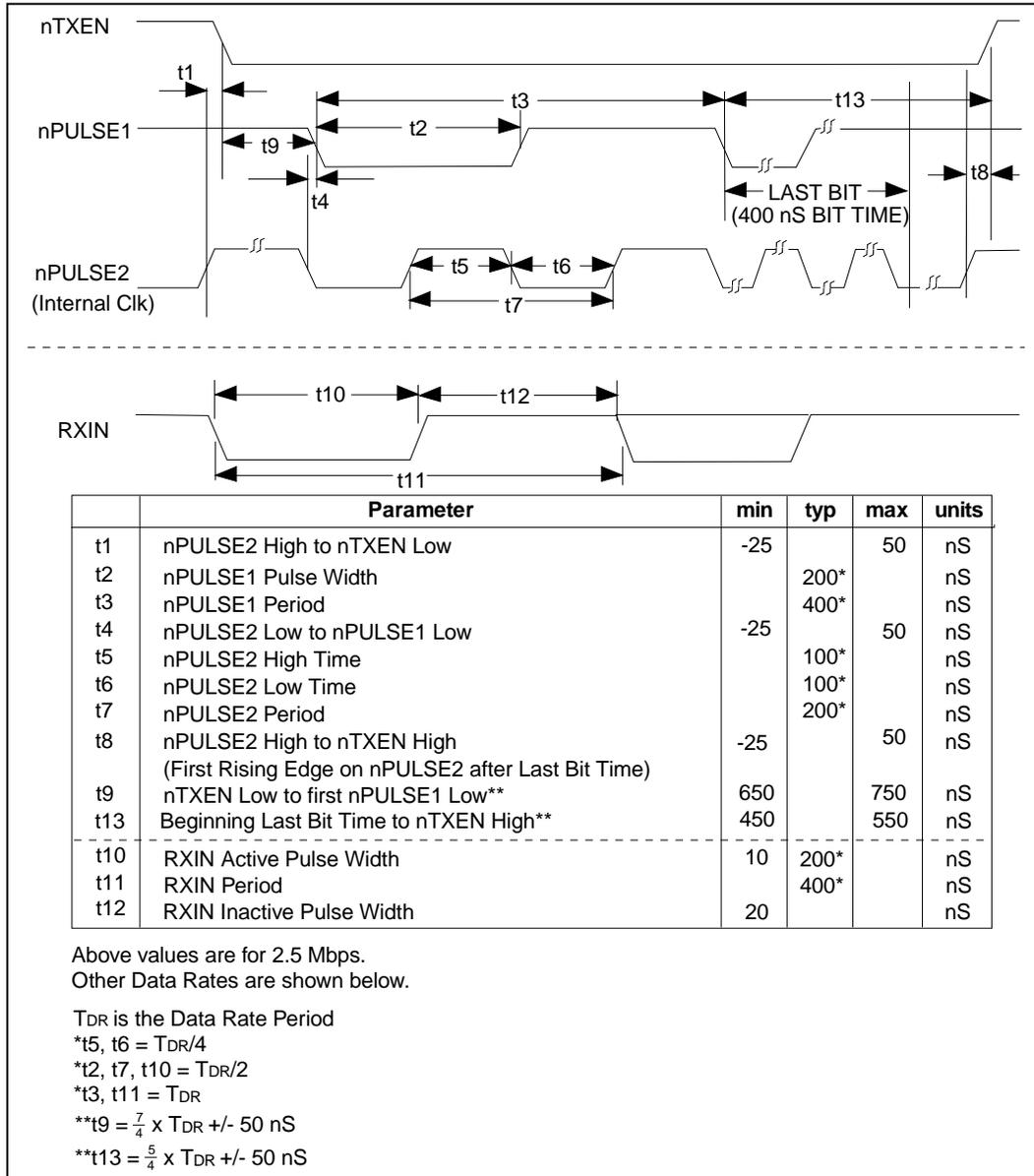
**Figure 24 – Backplane Mode Transmit or Receive Timing**
