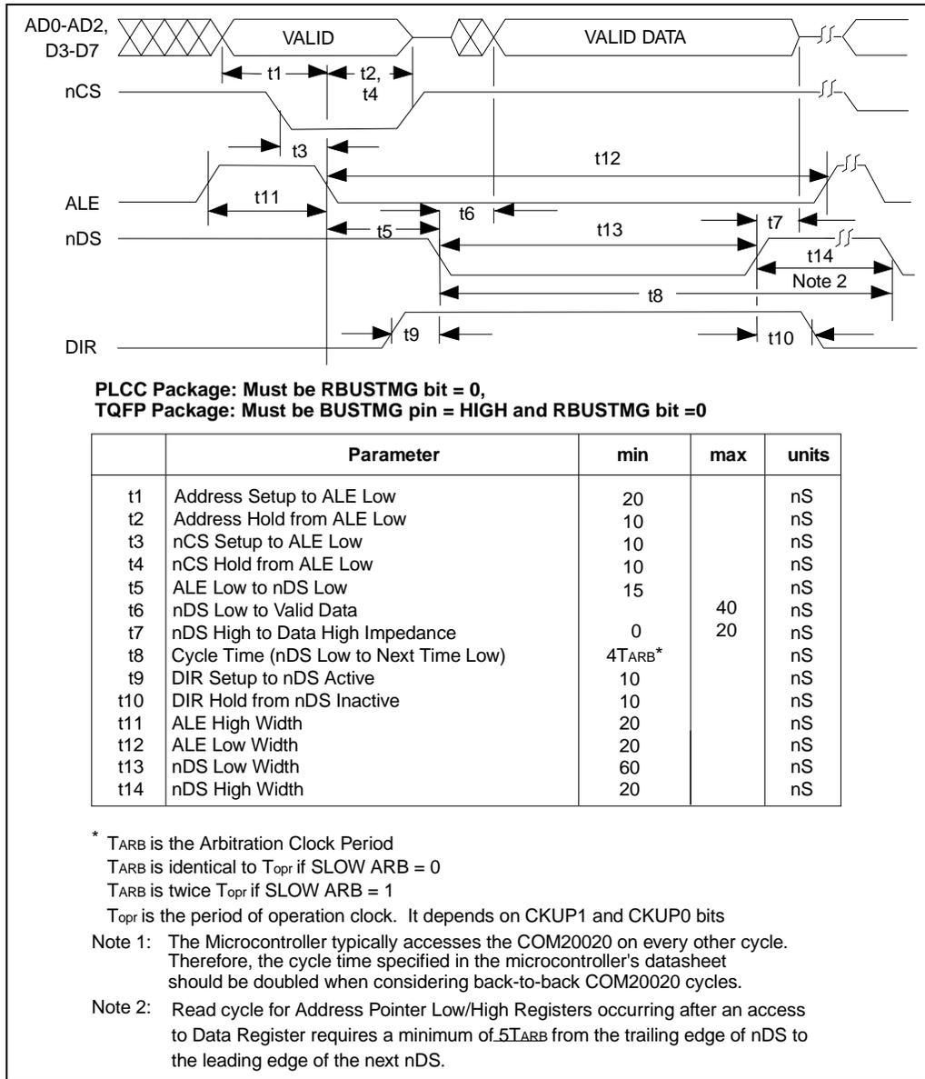
Figure 11 - Multiplexed Bus, 68xx-Like Control Signals; Read Cycle
