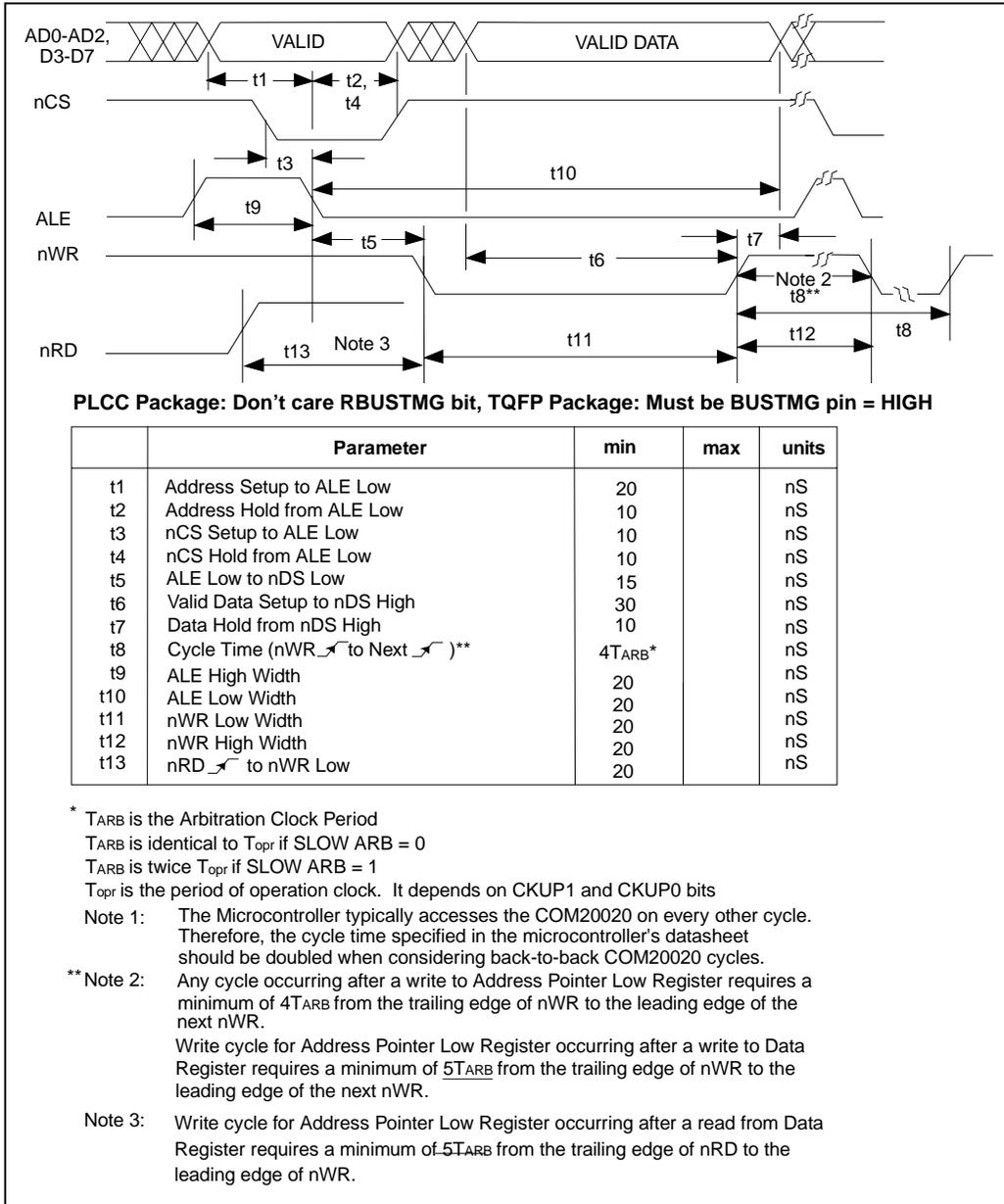
Figure 14 - Multiplexed Bus, 80xx-Like Control Signals; Write Cycle
