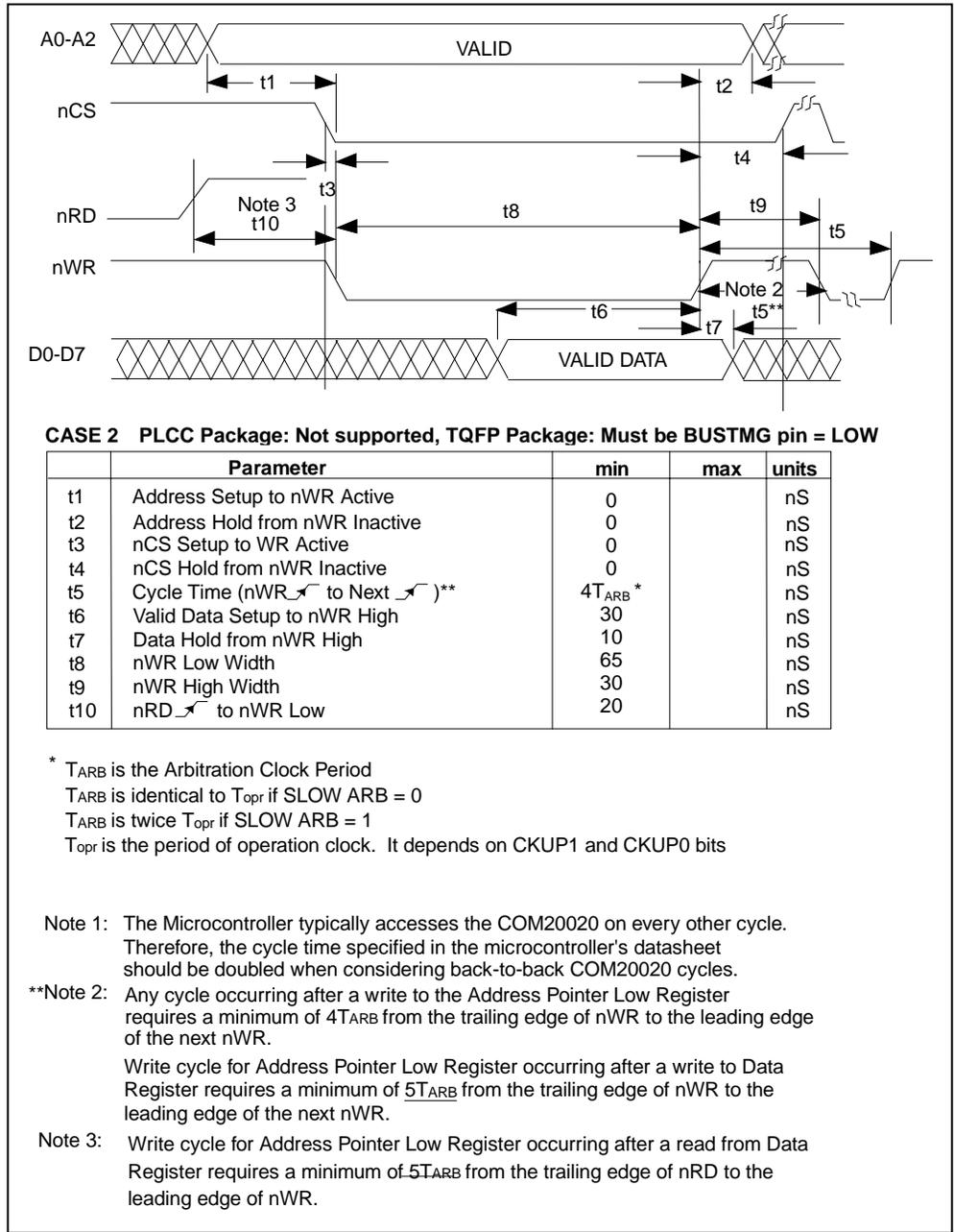
**Figure 20 - Non-Multiplexed Bus, 80xx-Like Control Signals; Write Cycle**
