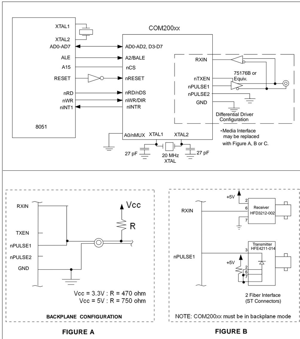
Figure 2 - Multiplexed, 8051-Like Bus Interface With RS-485 Interface
