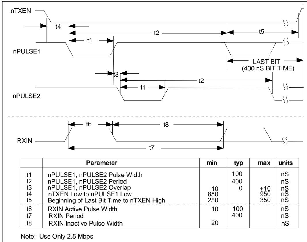
**Figure 23 – Normal Mode Transmit Or Receive Timing**
