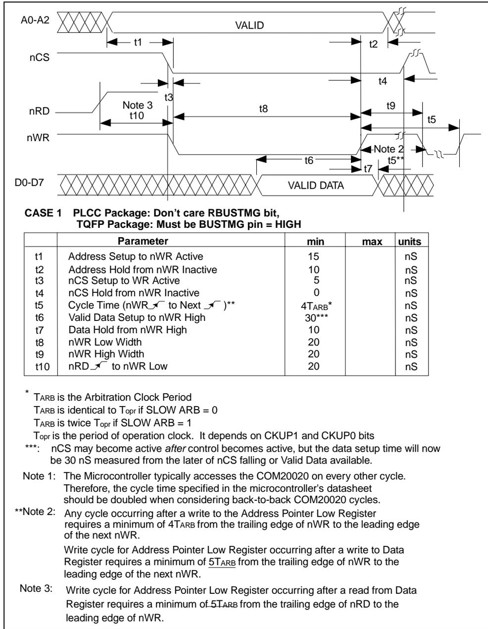
Figure 19 - Non-Multiplexed Bus, 80xx-Like Control Signals; Write Cycle
