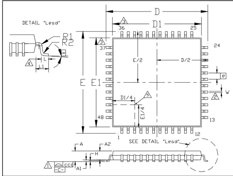
Figure 28 - 48 Pin TQFP Package Outline
