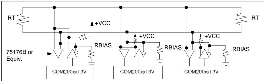
Figure 5 - COM20020I 3V Network Using RS-485 Differential Transceivers
