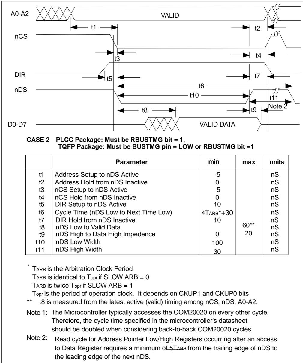
Figure 18 - Non-Multiplexed Bus, 68xx-Like Control Signals; Read Cycle
