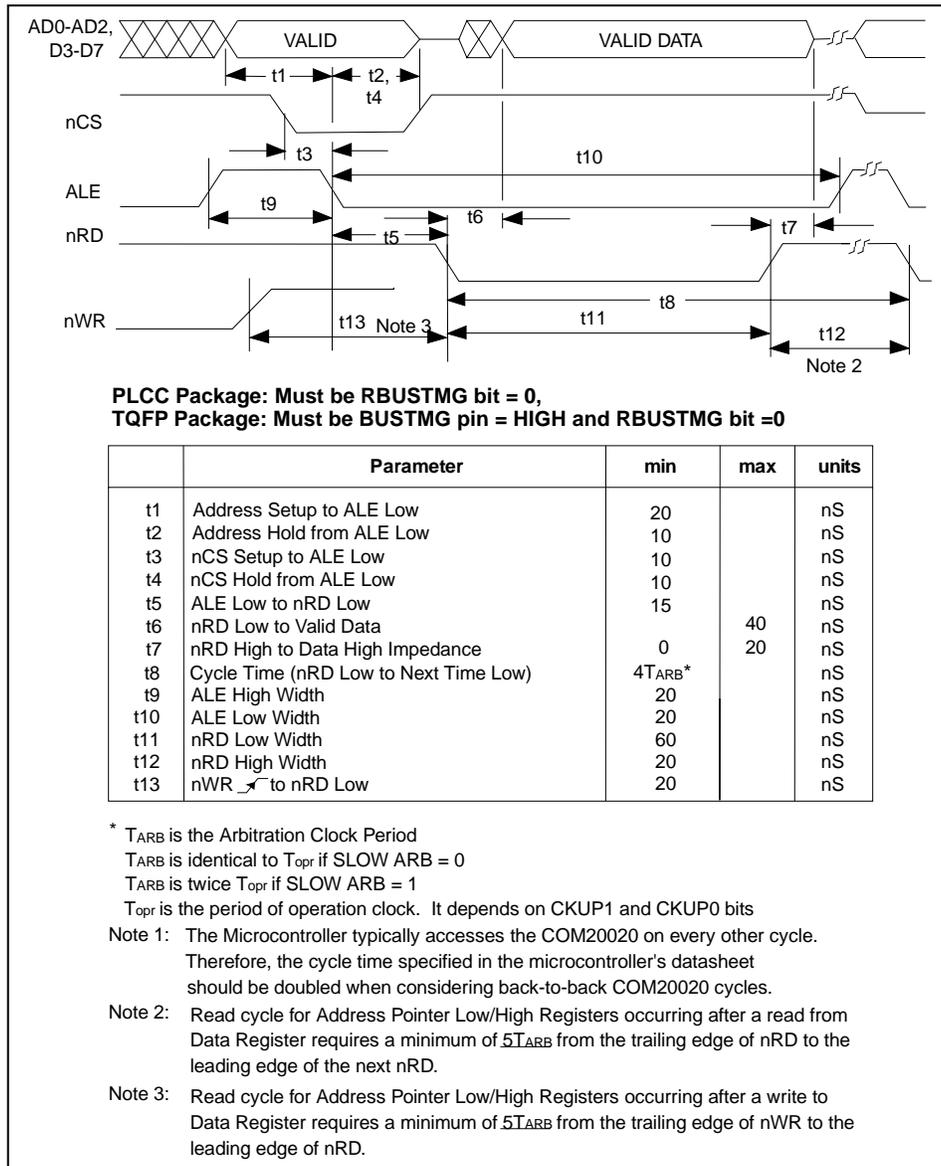
Figure 12 - Multiplexed Bus, 80xx-Like Control Signals; Read Cycle
