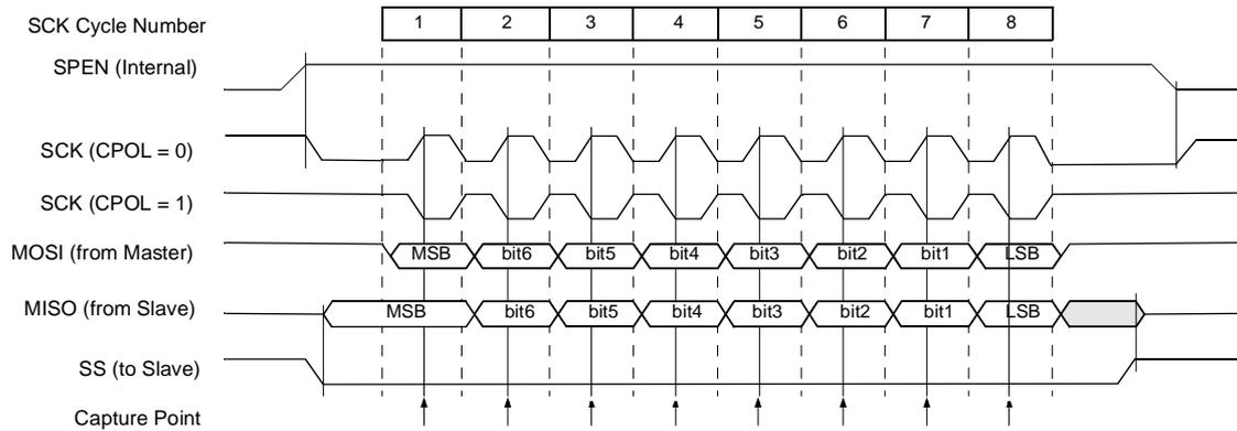
**Figure 29. Data Transmission Format (CPHA = 1)**
