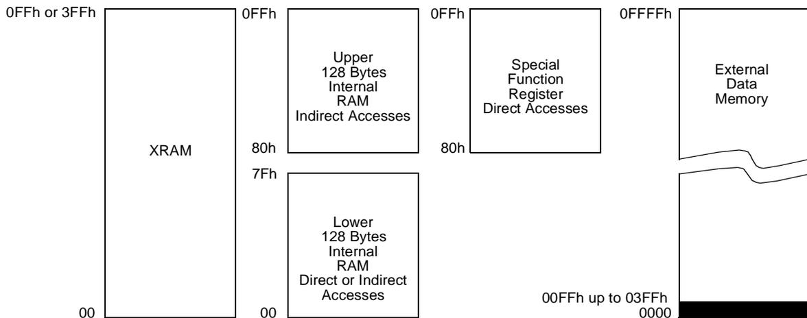
When an instruction accesses an internal location above address 7Fh, the CPU knows whether the access is to the upper 128 Bytes of data RAM or to SFR space by the addressing mode used in the instruction.
