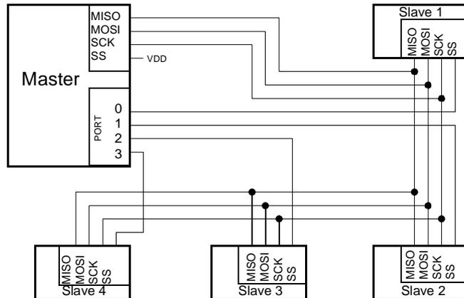
The Master device selects the individual Slave devices by using four pins of a parallel port to control the four  $\overline{SS}$  pins of the Slave devices.
