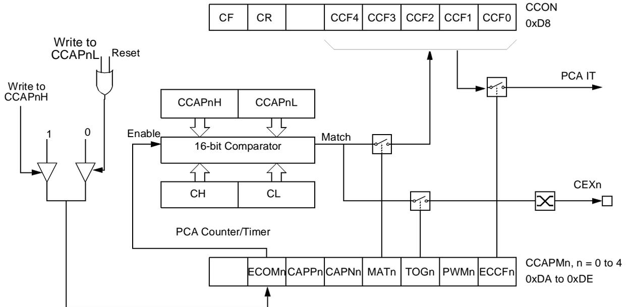
Before enabling ECOM bit, CCAPnL and CCAPnH should be set with a non-zero value, otherwise an unwanted match could occur.
