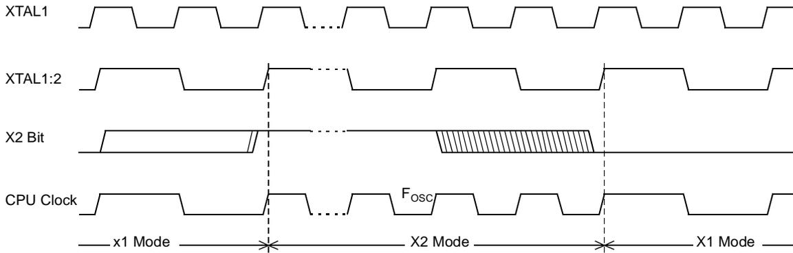
The X2 bit in the CKCON0 register (see Table 15) allows a switch from 12 clock periods per instruction to 6 clock periods and vice versa. At reset, the speed is set according to X2 bit of Hardware Security Byte (HSB). By default, Standard mode is active. Setting the X2 bit activates the X2 feature (X2 mode).
