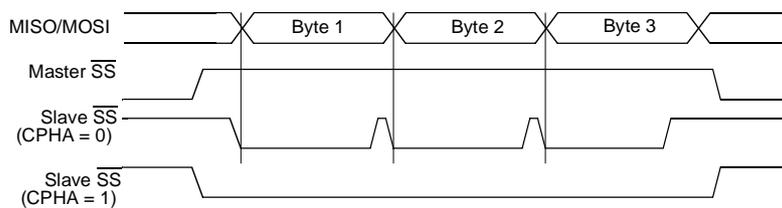
As shown in Figure 28, the first SCK edge is the MSB capture strobe. Therefore, the Slave must begin driving its data before the first SCK edge, and a falling edge on the  $\overline{SS}$  pin is used to start the transmission. The  $\overline{SS}$  pin must be toggled high and then low between each Byte transmitted (Figure 30).
