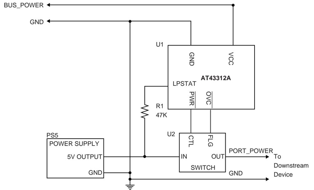
**Figure 3. Bus Powered Hub Power Supply**
