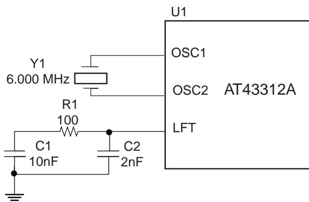
For proper operation of the PLL, an external RC filter consisting of a series RC network of 100Ω and 10 nF in parallel with a 2 nF capacitor must be connected from the LFT pin to VSS.
