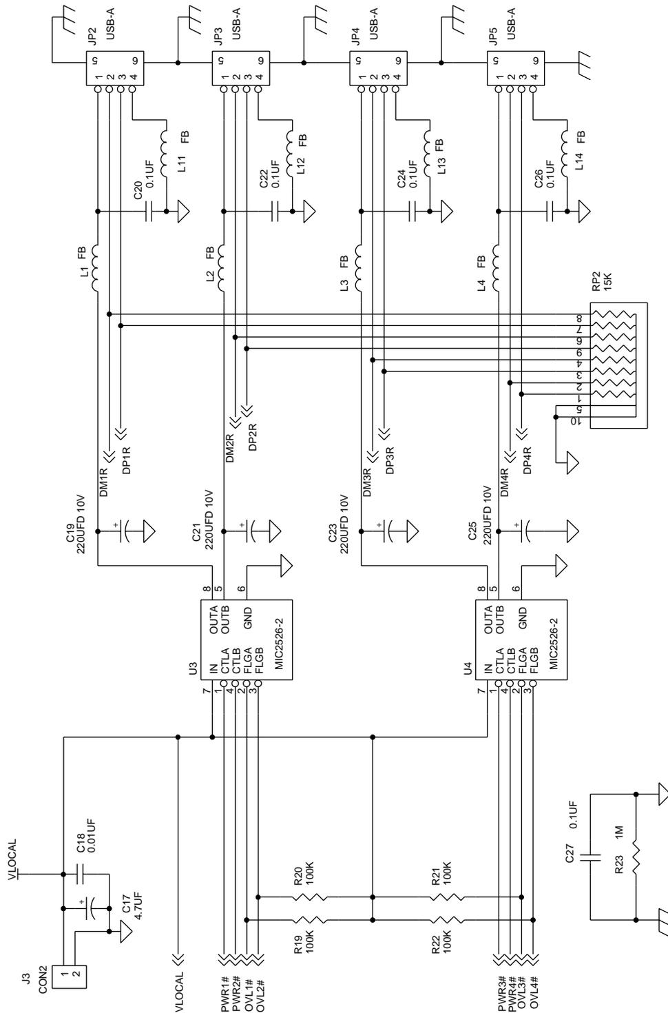
Figure 15. AT43312A Bus-powered USB Hub
