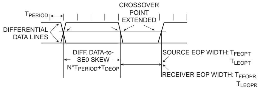
Figure 10. Receiver Jitter Tolerance
