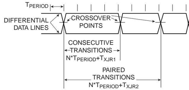
Figure 9. Differential-to-EOP Transition Skew and EOP Width
