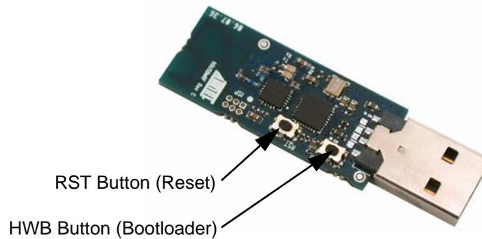
To force the execution the on-chip DFU bootloader, execute the following procedure:
