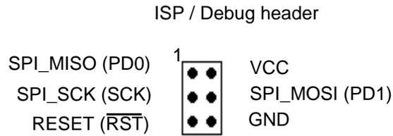
Note: The ISP / Debug header is not mounted by default, you need to solder a 1.27 pitch header on the board to be able to debug your firmware.
