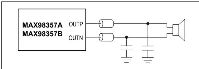
Figure 2. Optional Ferrite Bead Filter
