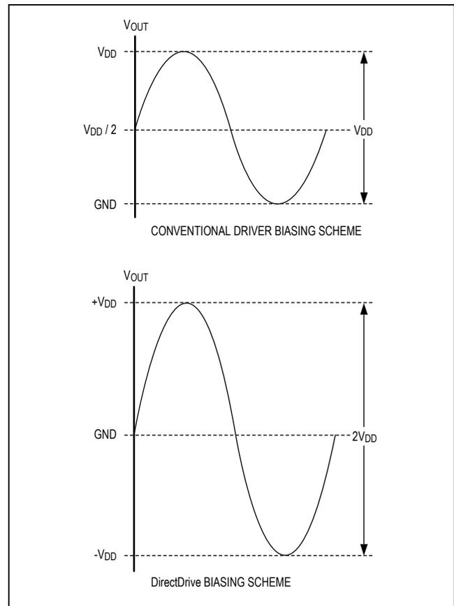
Figure 1. Traditional Amplifier Output vs. MAX9729 DirectDrive Output
