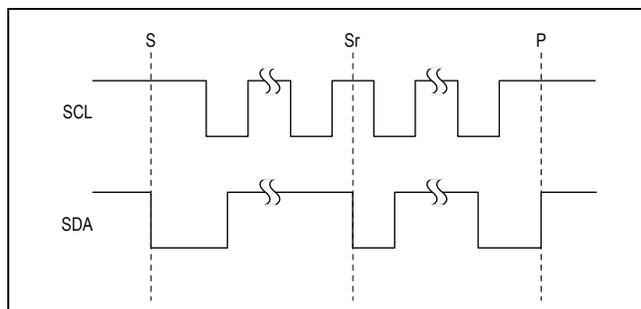
Figure 4. START, STOP, and REPEATED START Conditions
