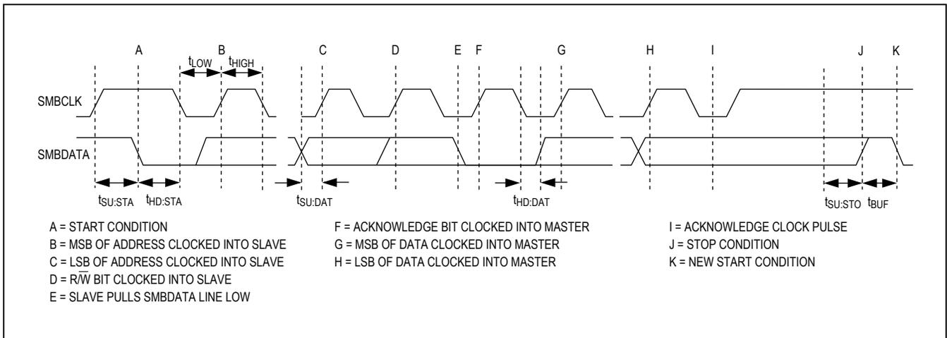
Figure 4. Read-Timing Diagram
