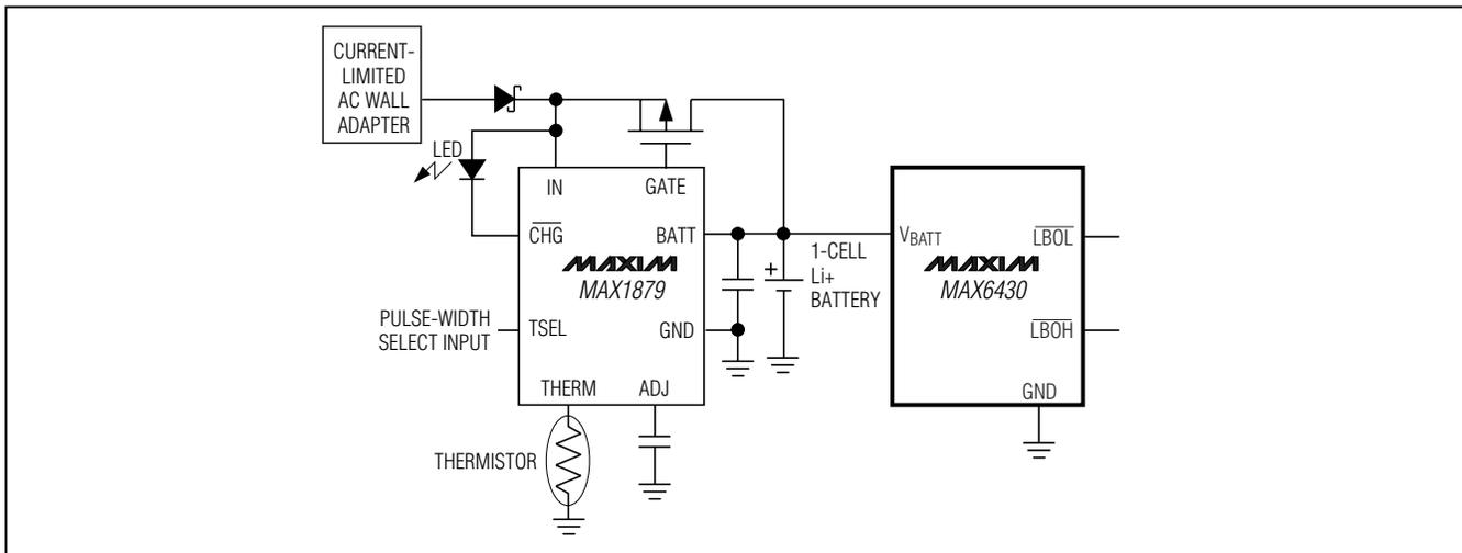
Figure 10. Lithium-Ion Cell Charger Application (using MAX1879)
