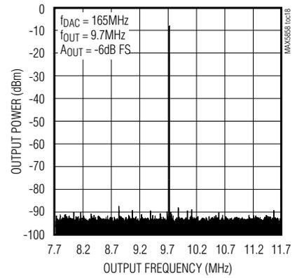
**FFT PLOT FOR NYQUIST WINDOW (NO INTERPOLATION,  $f_{DAC} = 165MHz$ ,  $f_{OUT} = 10MHz$ ,  $A_{OUT} = 0dB$  FS)**
