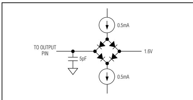
Figure 1. Load Test Circuit for CLK Outputs
