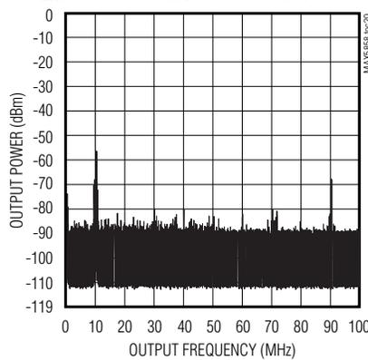
**FFT PLOT FOR DAC UPDATE NYQUIST WINDOW (100MHz) (4x INTERPOLATION,  $f_{DAC} = 200MHz$ ,  $f_{OUT} = 10MHz$ ,  $A_{OUT} = 0dB$  FS)**
