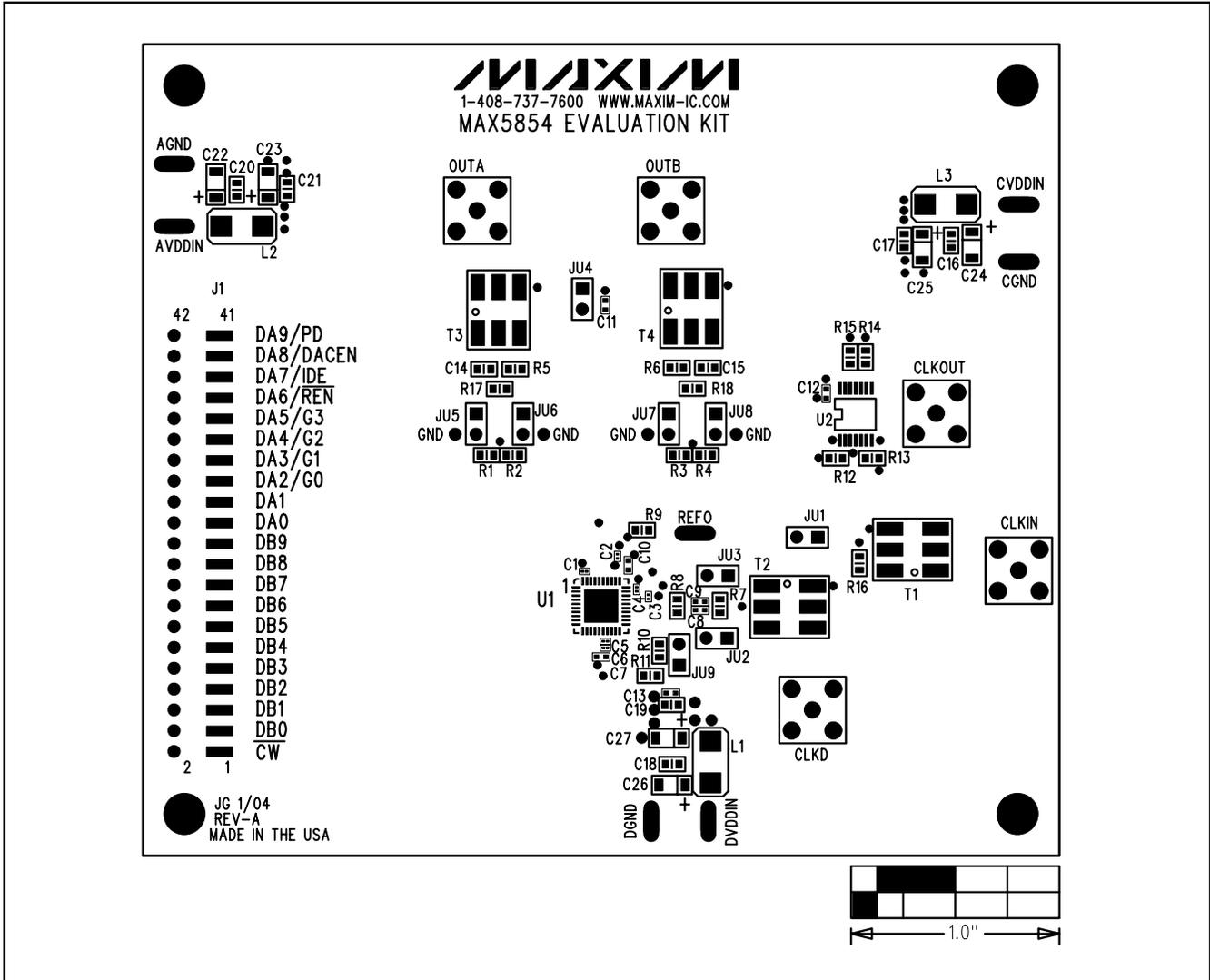
Figure 3. MAX5854 EV Kit Component Placement Guide—Component Side
