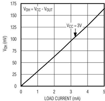
**OUTPUT-VOLTAGE LOW vs. LOAD CURRENT**
