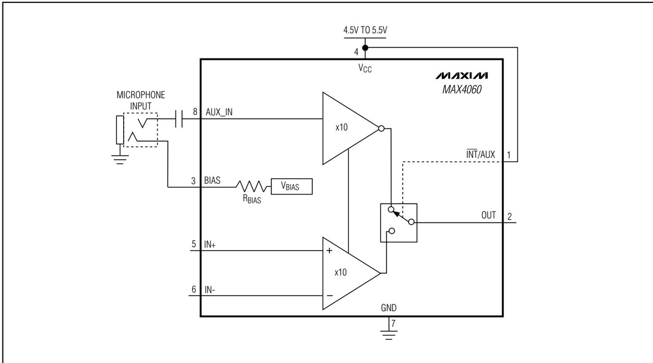
Figure 2. MAX4060 Used for Biasing a Microphone
