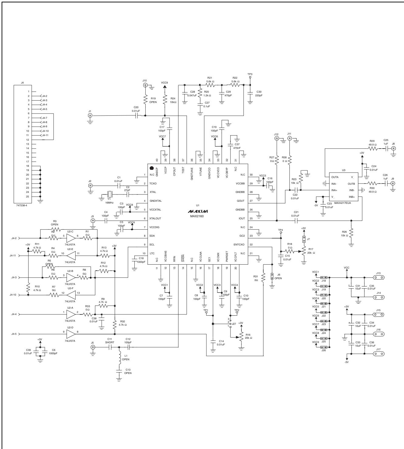
Figure 1. MAX2160 EV Kit Schematic
