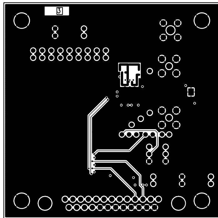
Figure 5. MAX2160 EV Kit PC Board Layout—Inner Layer 3
