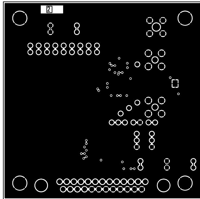
Figure 4. MAX2160 EV Kit PC Board Layout—Inner Layer 2
