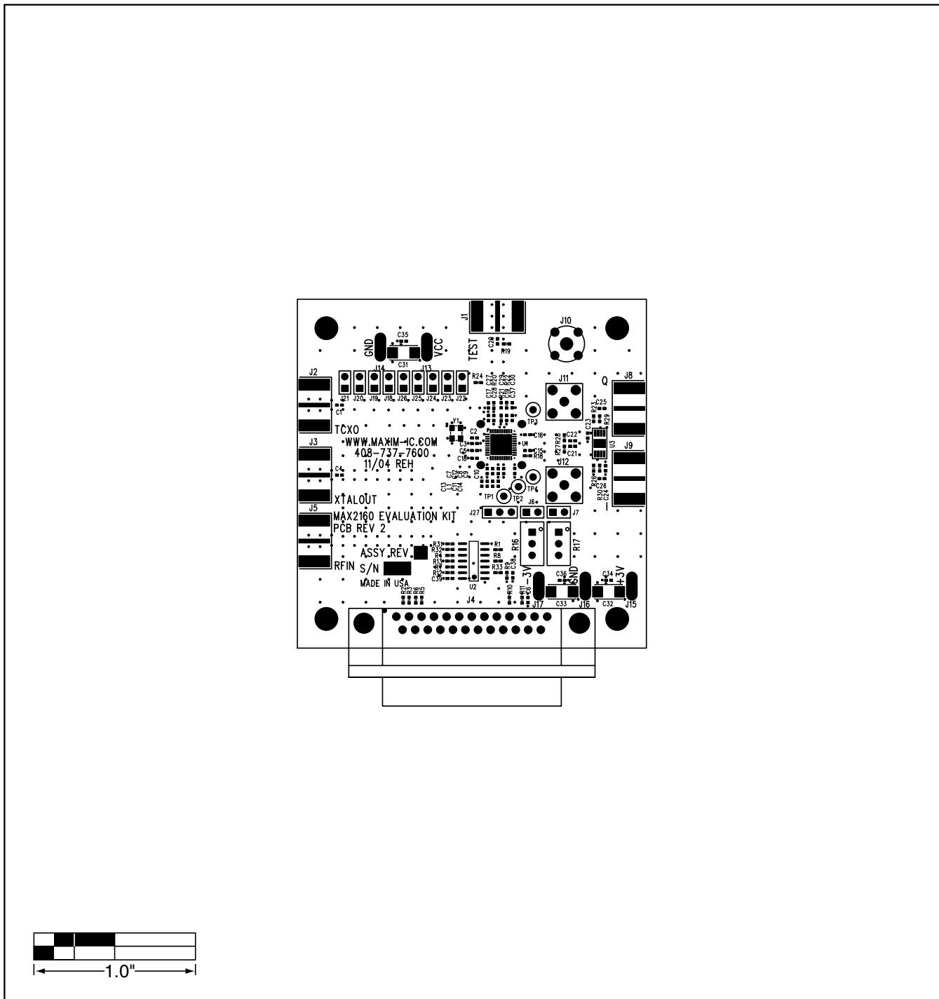
Figure 2. MAX2160 EV Kit PC Board Layout—Component Placement Guide
