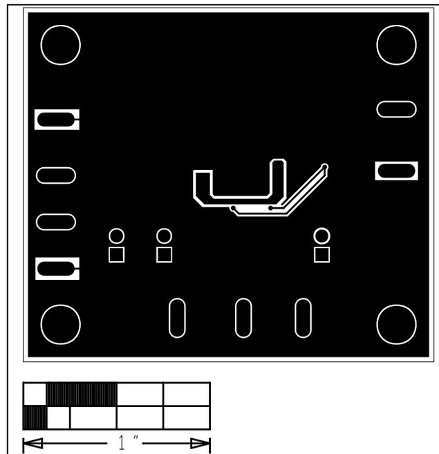
Figure 3. MAX17532 5V EV Kit (μMAX) PCB Layout—Solder Side
