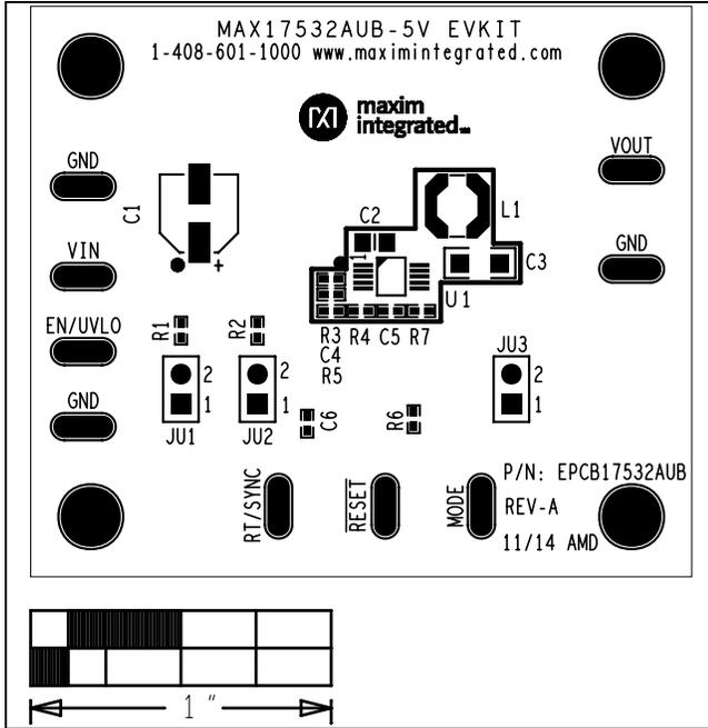
Figure 1. MAX17532 5V EV Kit (μMAX) Component Placement Guide—Component Side
