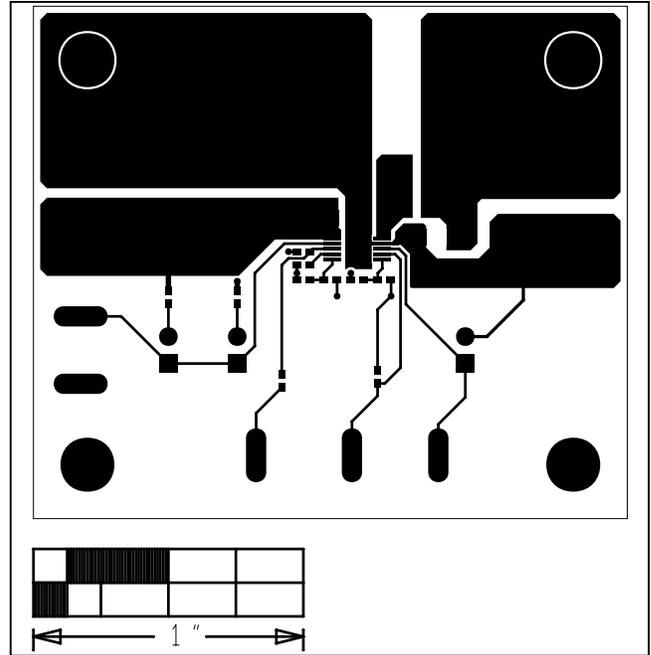
Figure 2. MAX17532 5V EV Kit (μMAX) PCB Layout—Component Side
