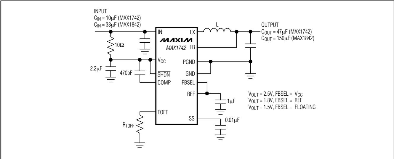
Figure 1. Typical Circuit
