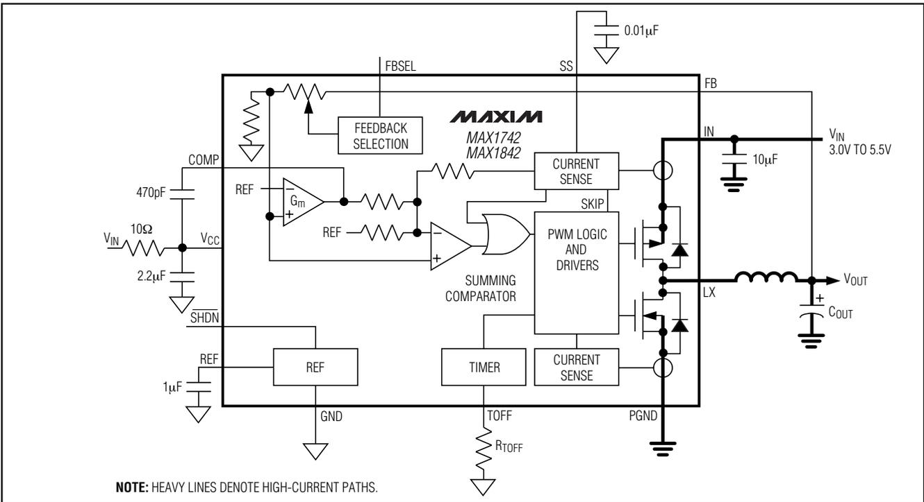
Figure 2. Functional Diagram
