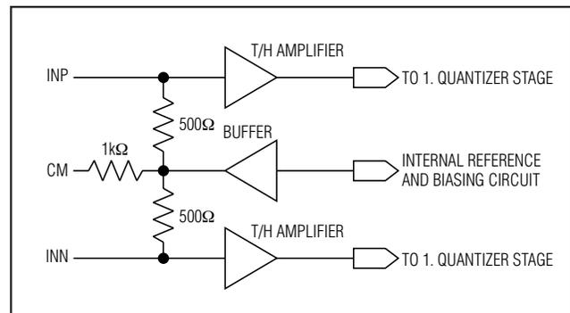
Figure 2. Simplified Analog and Common-Mode Input Architecture
