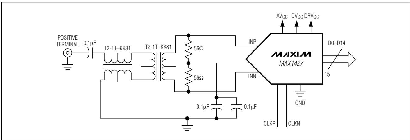
Figure 7. Transformer-Coupled Analog Input Configuration with Primary-Side Transformer
