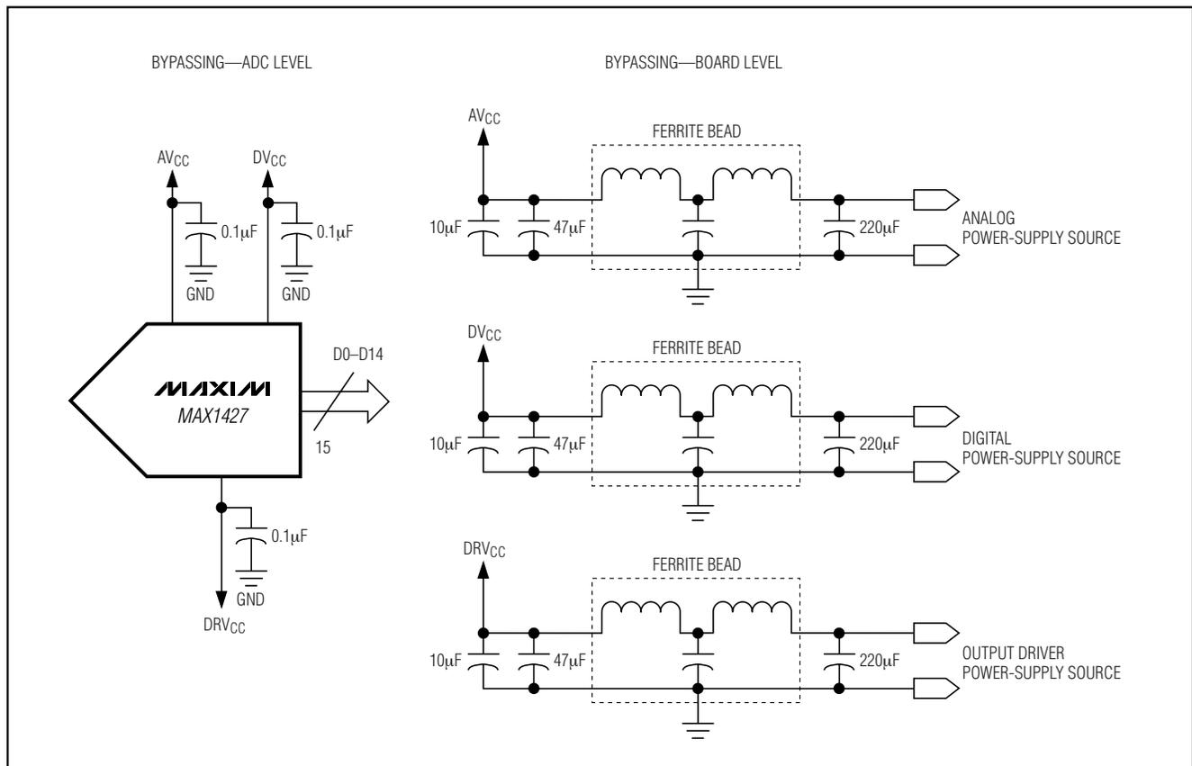
Figure 9. Grounding, Bypassing, and Decoupling Recommendations for MAX1427
