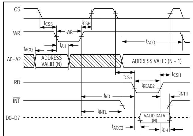
Figure 4. Write-Read Mode Timing ( $t_{RD} > t_{INTL}$ ) (Mode = 1)
