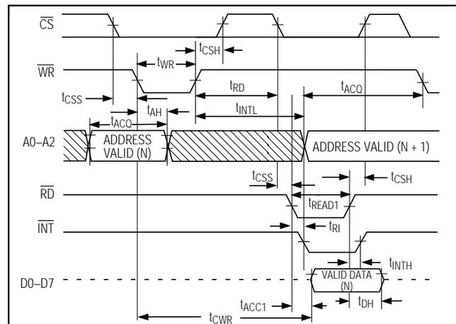
Figure 5. Write-Read Mode Timing ( $t_{RD} < t_{INTL}$ ) (Mode = 1)
