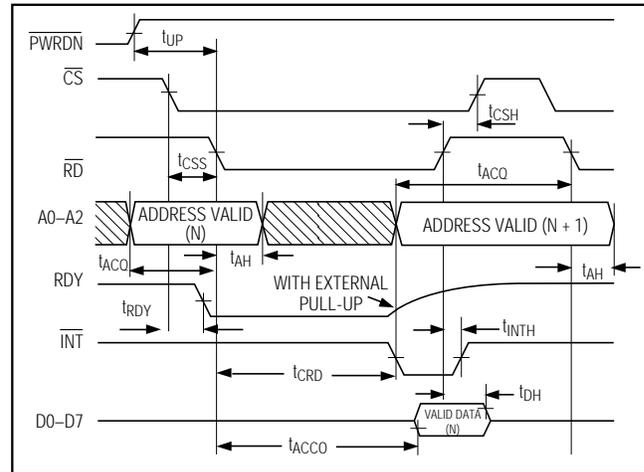
Figure 3. Read Mode Timing (Mode = 0)
