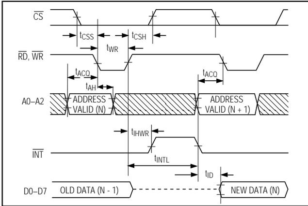
Figure 6. Pipelined Mode Timing ( $\overline{WR} = \overline{RD}$ ) (Mode = 1)
