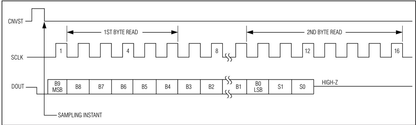
Figure 8c. SPI/MICROWIRE Interface Timing Sequence (CPOL = CPHA = 0)
