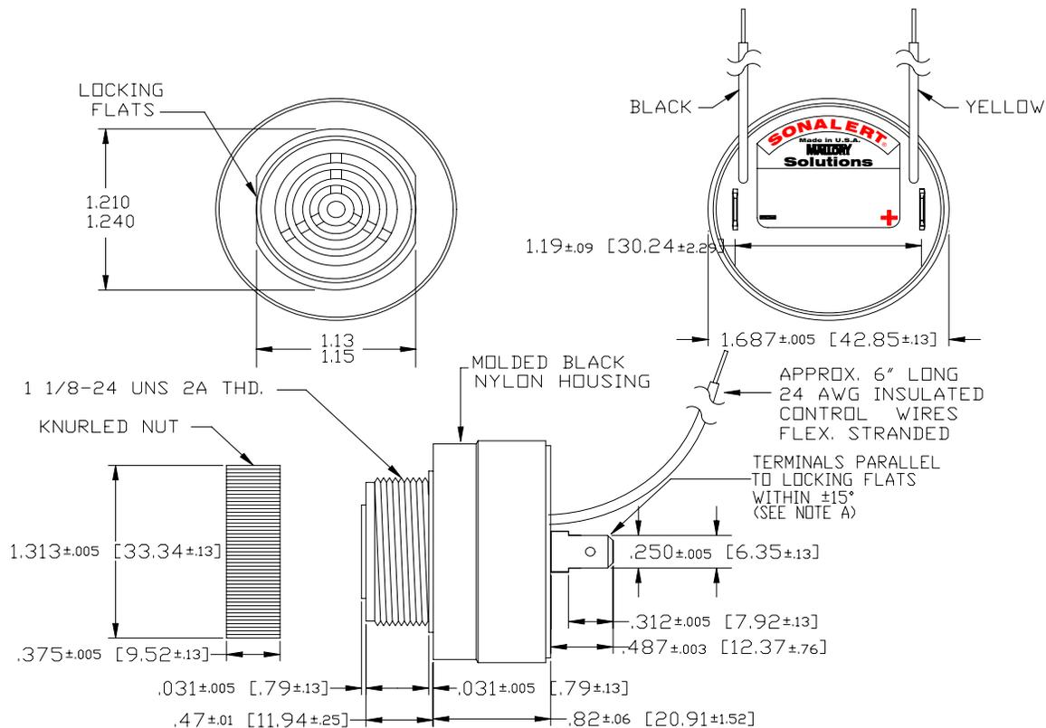
MOUNTING: REMOVE BLACK PLASTIC NUT AND INSERT THREADED FRONT THROUGH 1.25" HOLE PUNCHED IN PANEL, IF ORIENTATION IS NEEDED, NOTE LOCKING FLATS ON DRAWING. SCREW NUT BACK ON. DO NOT OVERTIGHTEN.
