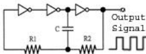
The capacitor and resistors values need to be set to provide a signal at the appropriate rated buzzer frequency. For example, if the electromagnetic buzzer is rated at 2.3 KHz, then the output signal's frequency from the microcontroller or from the above circuit needs to be at 2.3 KHz.
