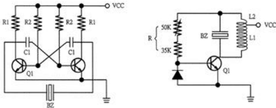
The following three circuits provide a means to drive the electromagnetic transducer buzzer, but they require an input signal to turn the drive circuitry off and on at the appropriate rated buzzer frequency. Care must be taken not to over-voltage the buzzer.
