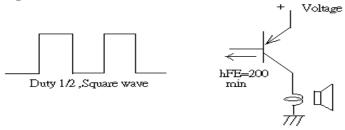
The base current Ib should be high enough so that it saturates the collector current of the transistor with the CB load.
