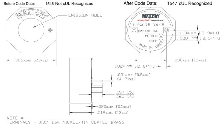
MOUNTING- INSERT INTO PRINTED CIRCUIT BOARD AND HAND OR MACHINE SOLDER, UNITS ARE SUITABLE FOR WAVE SOLDERING. BOARDS ARE NOT SUITABLE FOR WASH, RECOMMENDED MAXIMUM TEMPERATURE AND TIME DURATION FOR WAVE SOLDERING IS
