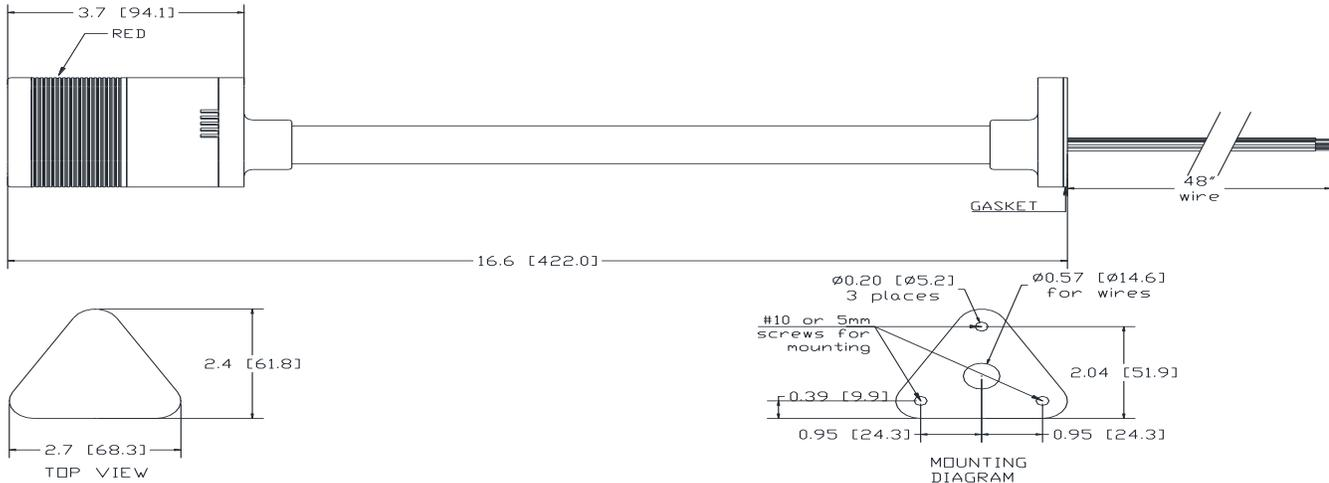
**LED OPERATION:** CONNECT STACK COLOR WIRE TO POWER AND BROWN WIRE TO POWER.
