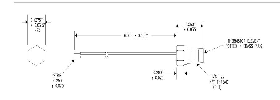
RESISTANCE @  $+25^{\circ}$ C = 10,000  $\Omega$  ± 5% RESISTANCE/TEMPERATURE CURVE = "J" TEMPERATURE COEFFICIENT @  $+25^{\circ}$ C = -4.4%/°C NOMINAL MAXIMUM TEMPERATURE RATING =  $+105^{\circ}$ C
