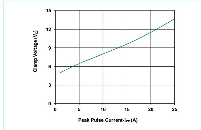
**Clamping Voltage vs. I<sub>pp</sub> (Line-to-Line)**
