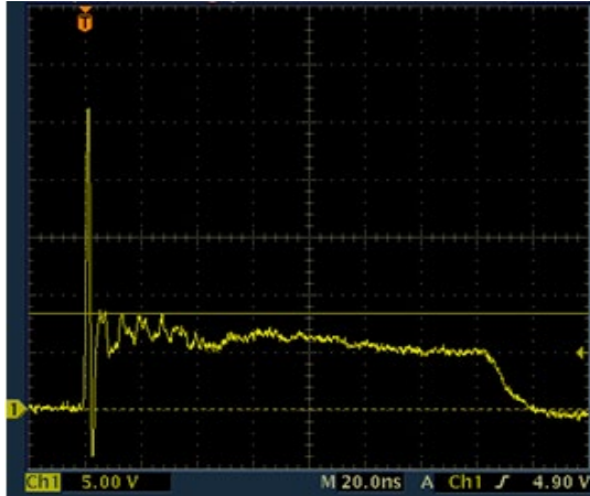
SP1105S IEC 61000 -4-2 +8 kV Contact ESD Clamping Voltage
