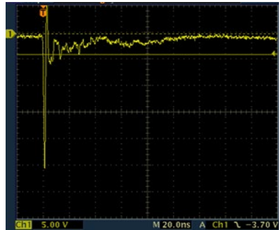
SP1112 IEC 61000 -4-2 -8 kV Contact ESD Clamping Voltage
