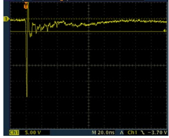
SP1105S IEC 61000 -4-2 -8 kV Contact ESD Clamping Voltage
