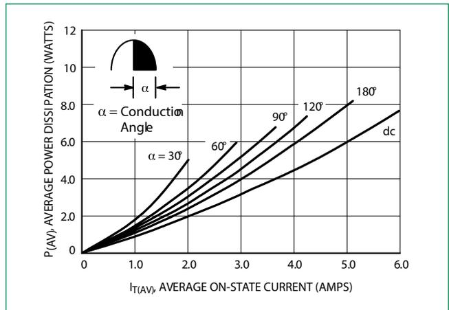
**Figure 3. On-State Characteristics**
