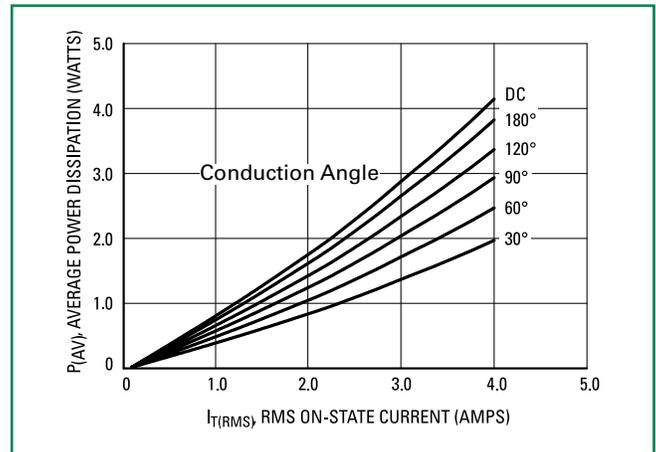
Figure 3. On-State Characteristics
