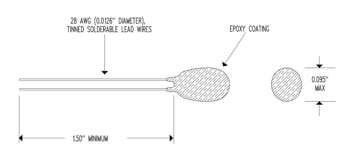
RESISTANCE @ +25°C = 3,000  $\Omega$  ± 5% RESISTANCE/TEMPERATURE CURVE = "J" TEMPERATURE COEFFICIENT @ +25°C = -4.4%/°C NOMINAL BETA " $\beta$ " (0 TO +50°C) = 3,892°K NOMINAL DISSIPATION CONSTANT = 1 mW/°C NOMINAL THERMAL TIME CONSTANT = 10 SECONDS MAXIMUM (STILL AIR) THERMAL TIME CONSTANT = 1 SECOND MAXIMUM (WELL STIRRED OIL) MAXIMUM TEMPERATURE RATING = +150°C
