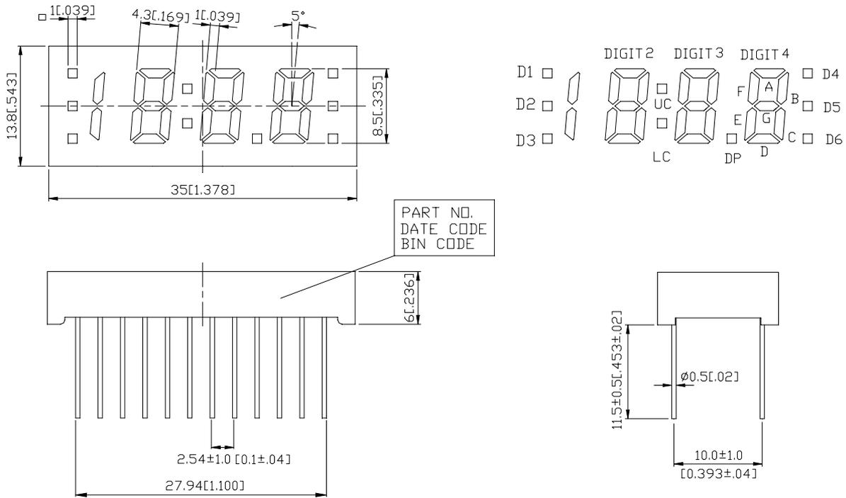
NOTES: All dimensions are in millimeters. Tolerances are ± 0.25 mm (0.01") unless otherwise noted.
